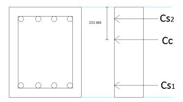
$$M = C_c * \left(\frac{250 - 233.484}{1000}\right) + C_{s2} * 0.15 - C_{s1} * 0.15 = 131.232 \text{ KNM}$$
