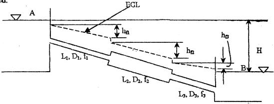
For datum through B. the energy equation including the loss terms takes the form:
