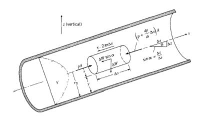
Consider a case of steady laminar flow in a circular pipe shown below:
