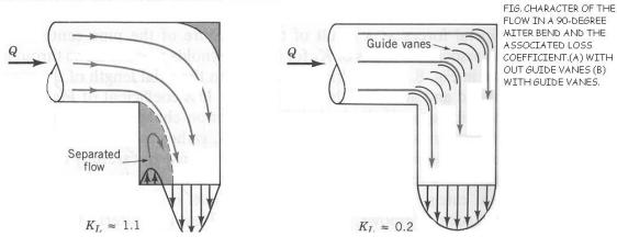
Loss Coefficients for Pipe Components  $\left(h_L = K_L \frac{V^2}{2g}\right)$
