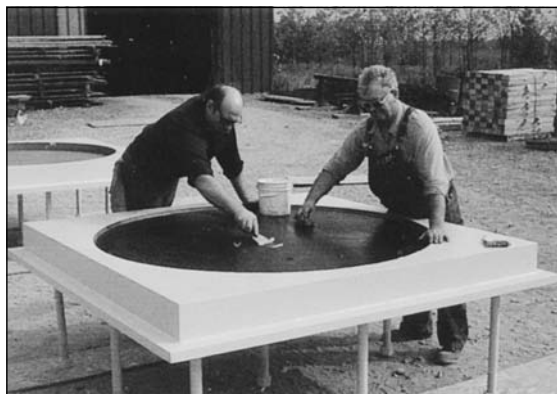
Figure 4.17 Workers assemble a 12,000,000 pound capacity pot bearing for the State of Florida. (Photograph courtesy of D. S. Brown Company, North Baltimore, Ohio.)
