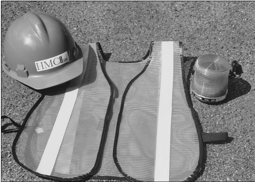
Figure 2.11 Three tools inspectors should always have.
