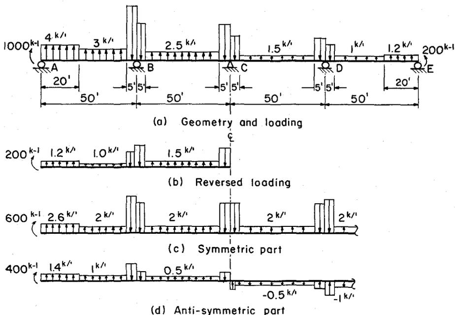
Fig. 4. 4-span structure with non-symmetric loading for Example 2
