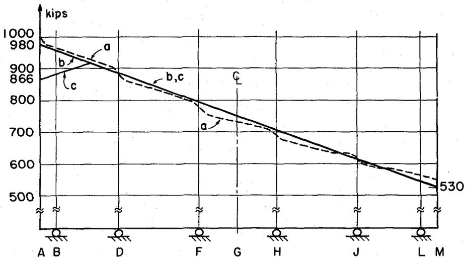
Fig. 10. Tendon force variation, jacking from one end
