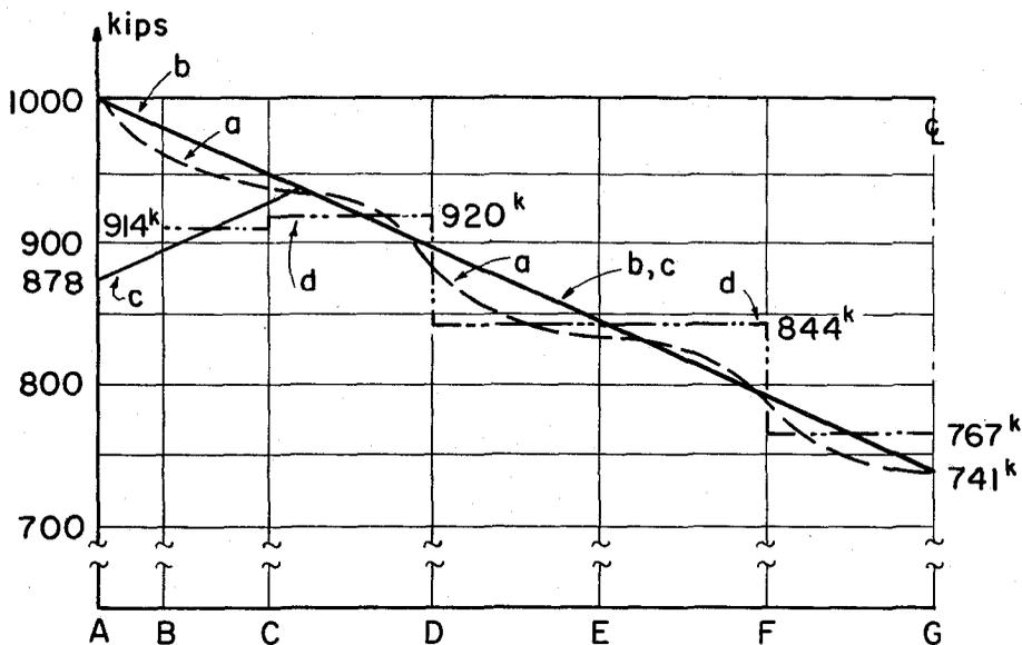
Fig. 8. Tendon force variation, jacking from both ends
