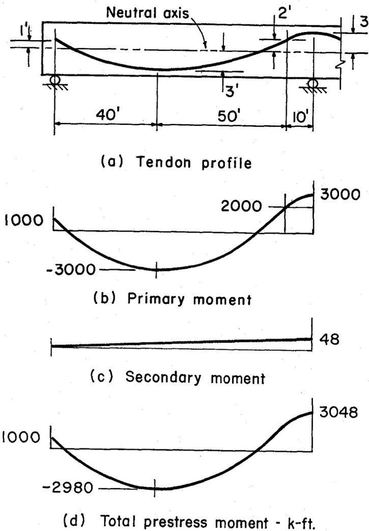
Fig. 6. Bending moments between supports for Example 4
