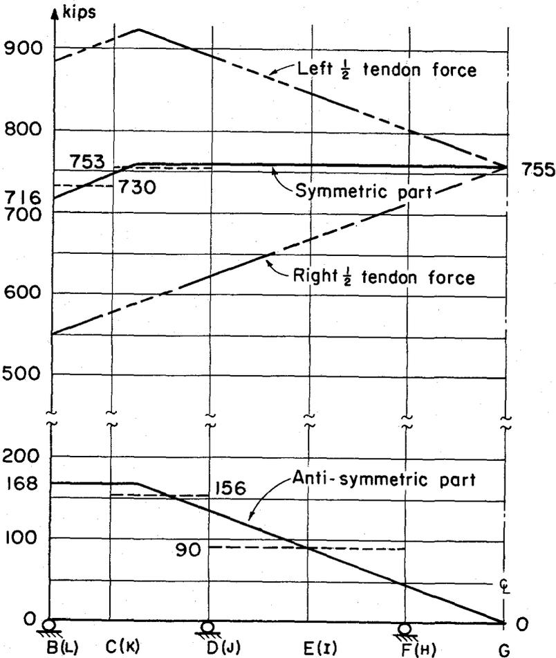
Fig. 11. Symmetric and anti-symmetric tendon forces for Example 6
