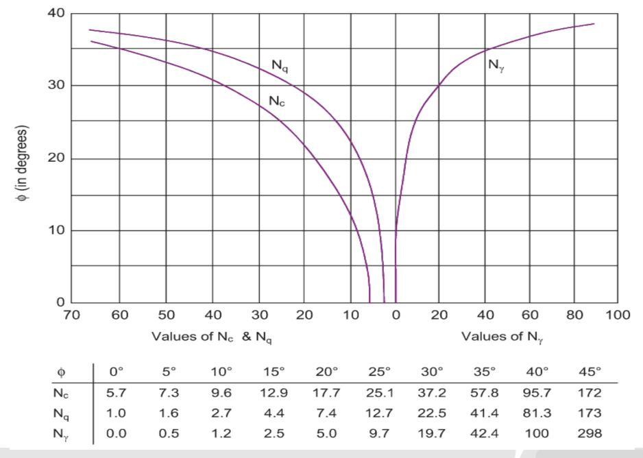
The increase in the value of Nc from 5.14 to 5.7 is due to the fact that Terzaghi allowed for frictional effects between the foundation and its supporting soil.
