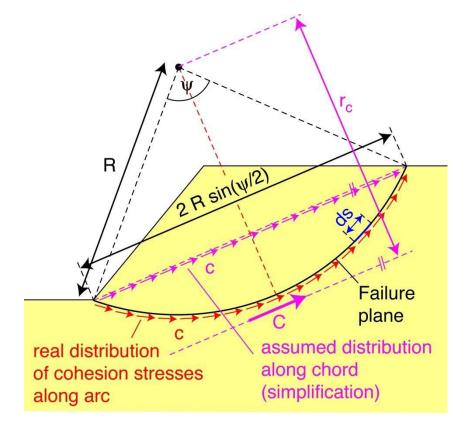
Failure analysis with slip circles is based on momentum equilibrium → it is important to consider the exact moment M<sub>c</sub>
