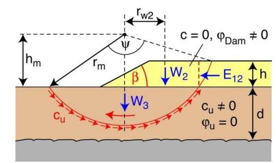
$$c_{u,\min} = \frac{\gamma_{\text{Dam}} \cdot h^2}{R^2 \cdot \psi} \cdot \left[ m_w \cdot n_w \cdot h + \frac{1}{2} \cdot \tan^2 \left( 45^\circ - \frac{\varphi_{\text{Dam}}}{2} \right) \cdot \left( h_m - \frac{h}{3} \right) \right]$$
