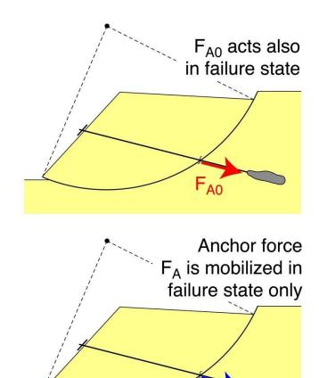
Non-prestressed anchors: F<sub>A</sub> is considered on the side of resisting moments (increasing)
