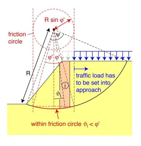
For  $\vartheta_i < \phi$  additional driving force and moment due to  $P_i$  is smaller than additional resisting force and moment due to  $P_i$
