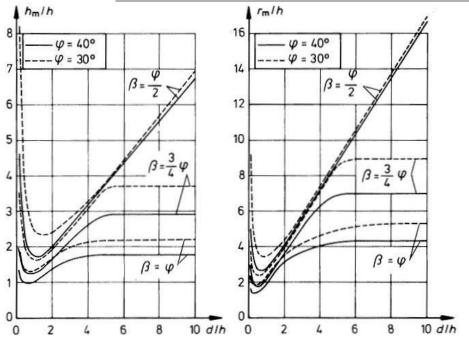
Can be used to estimate the maximum possible height h of embankment
