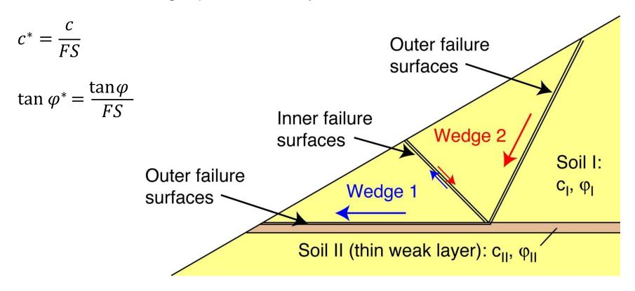
Example 1: Two wedges on weak soil layer
