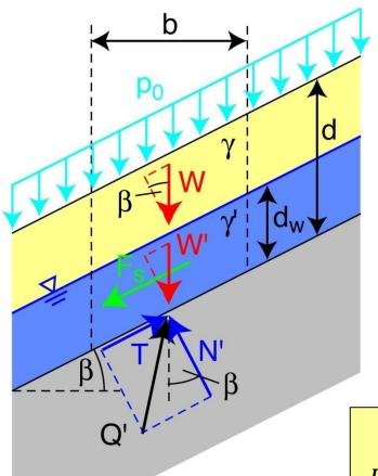
Resulting force due to surface load
