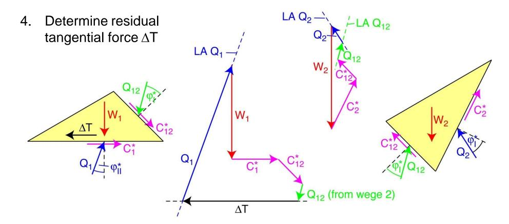
If  $\Delta T$  is acting in sliding direction  $\rightarrow$  safety is higher than estimated FS (additional  $\Delta T$  is necessary to cause failure)  $\rightarrow$  next iteration with higher FS until  $\Delta T \approx 0$
