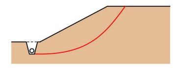
Excavation of soil in front of the toe of the slope, e.g. in order to install tubes, cables, etc.
