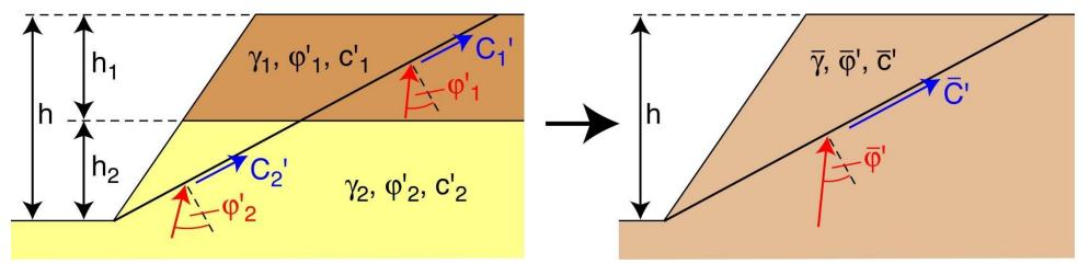
$$\gamma = \gamma_1 \cdot \left[ 1 - \left( \frac{h_2}{h} \right)^2 \right] + \gamma_2 \cdot \left( \frac{h_2}{h} \right)^2 \qquad \tan \varphi = \tan \varphi_1 \cdot \left( \frac{h_1}{h} \right)^2 + \tan \varphi_2 \cdot \left[ 1 - \left( \frac{h_1}{h} \right)^2 \right]$$
