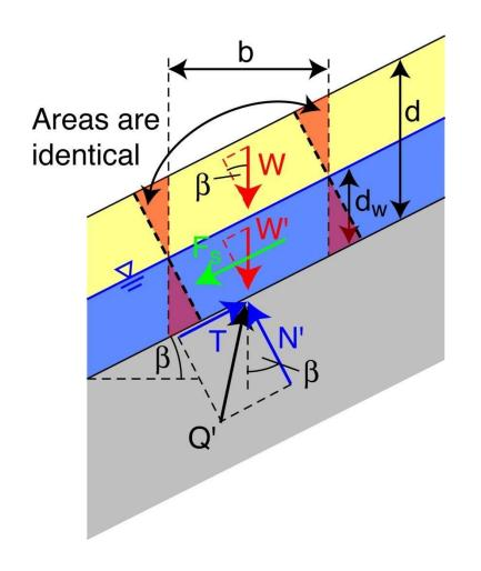
Comparison of bodies with boundaries being either vertical or perpendicular to the ground surface
