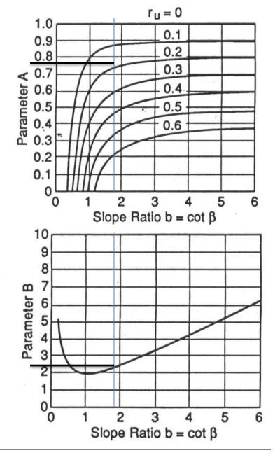
Water flow parallel to slope, soil with  $\varphi'$  and c'
