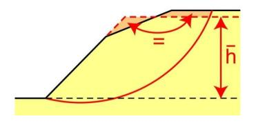
Analysis with substitutional height h, so that the sliding mass is identical for the original and the simplified geometry
