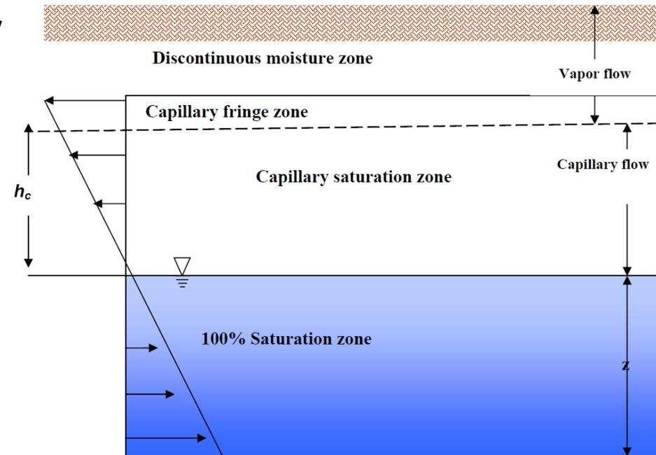
→ capillary is more pronounced in fine grained soils than in course grained .
