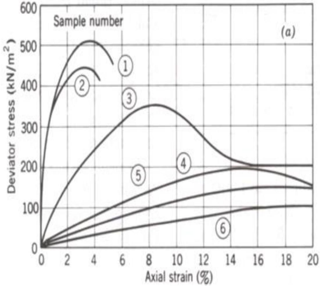
Samples compacted dry of optimum tend to be more rigid and stronger than samples compacted wet of optimum
