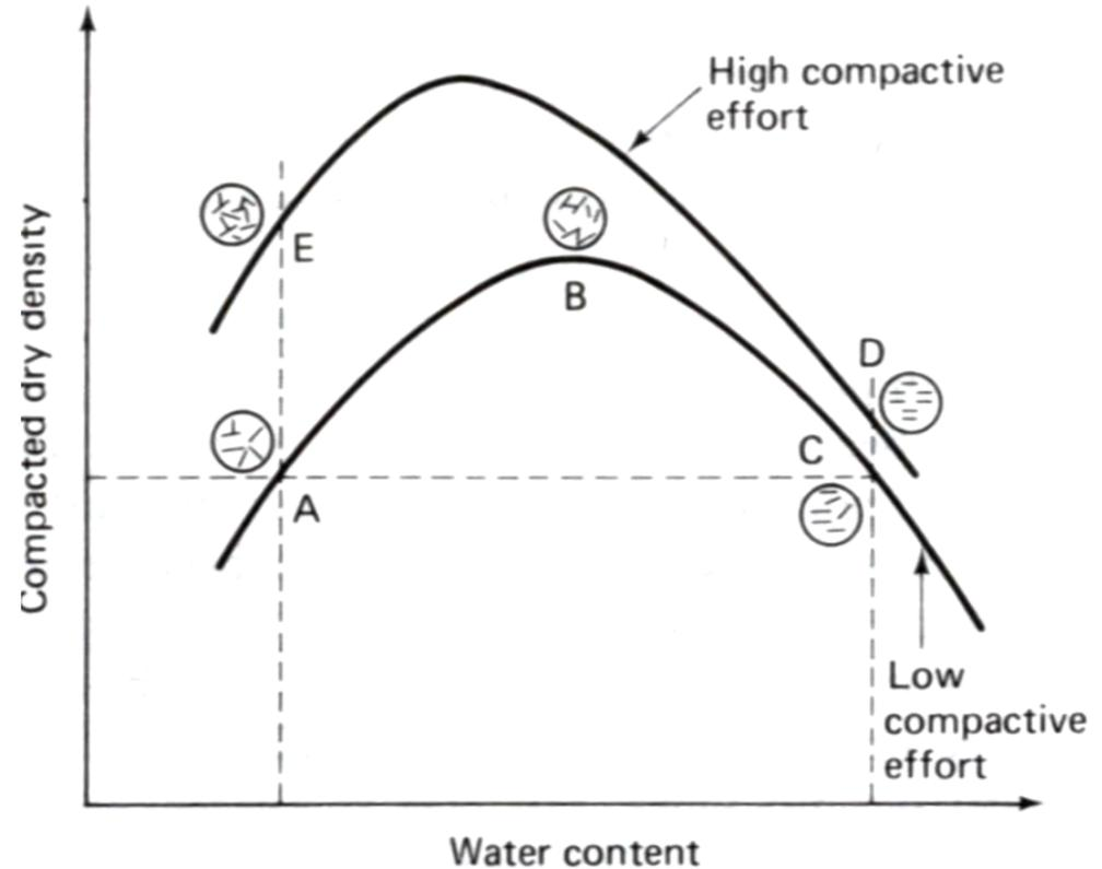
Effect of compaction on soil structure (after Lambe, 1958a).
