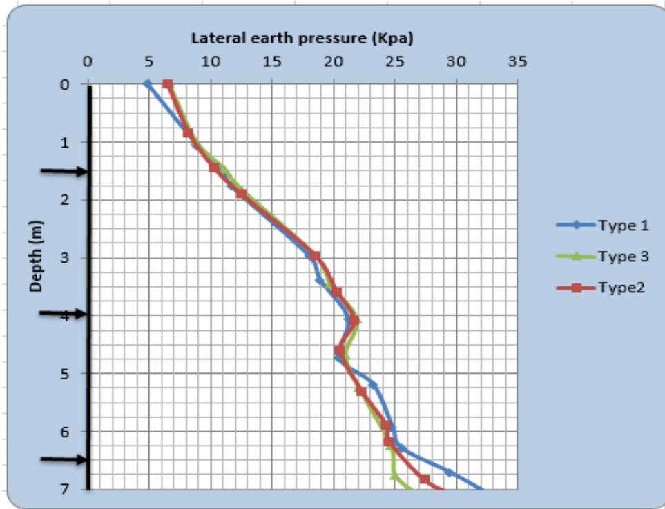
Figure 4-9: Lateral Earth pressure variation due to stiffness of sheet pile of sandy soil
