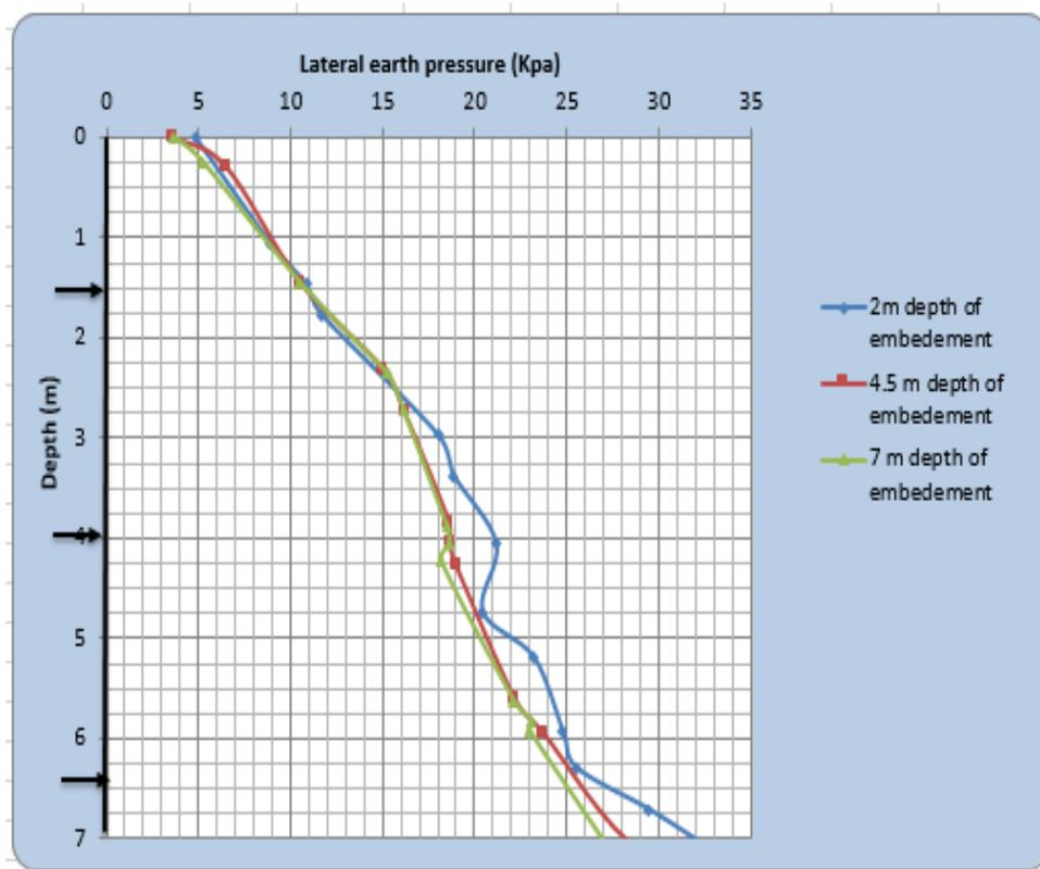
Figure 4-5: Lateral Earth pressure variation due to depth of embedment of sandy soil
