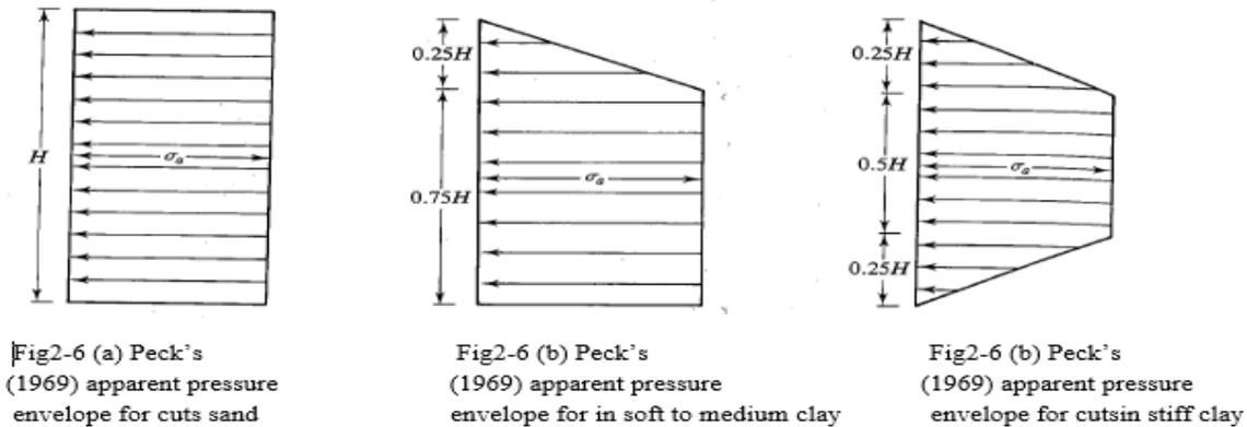
Figure 2-6 : Apparent pressure envelope of Peck (1969)
