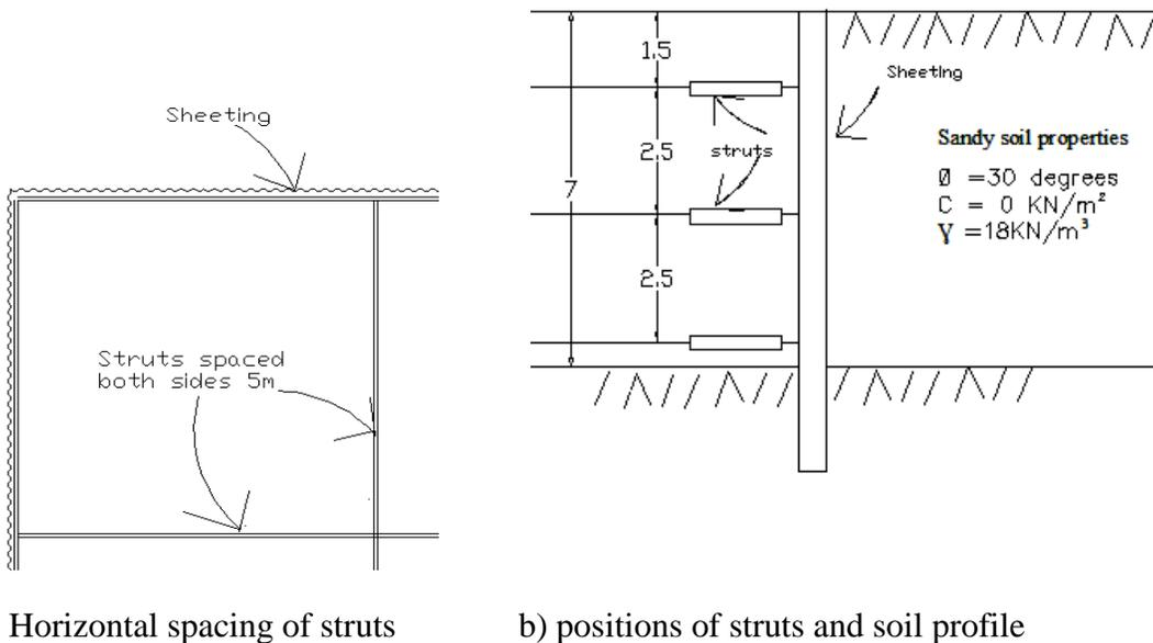
Figure 3-1: supporting system of braced excavation for sandy soil
