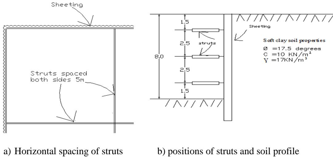
Figure 3-2: supporting system of braced excavation for soft clay soil
