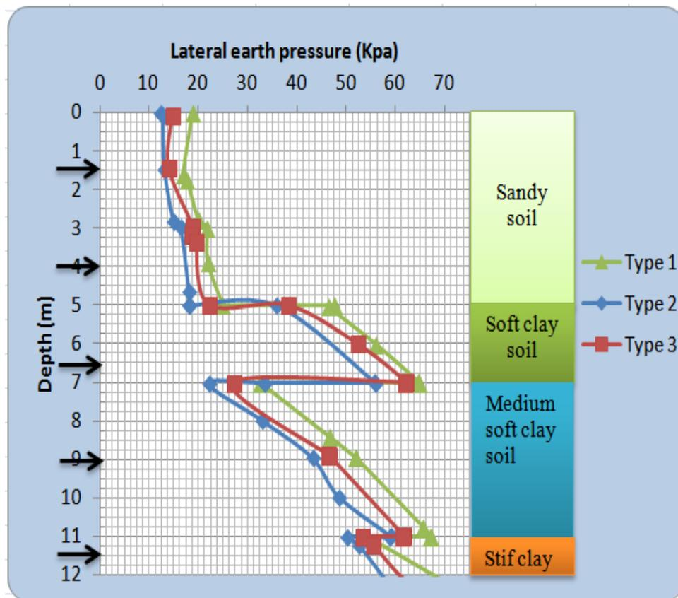
Figure 4-16: Lateral Earth pressure variation due to spacing of struts of stratified soil type 2
