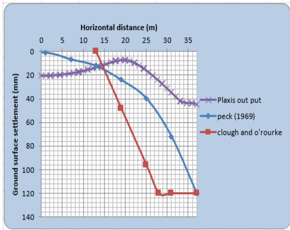
Figure 4-32: Ground surface settlement for stratified soil type 1
