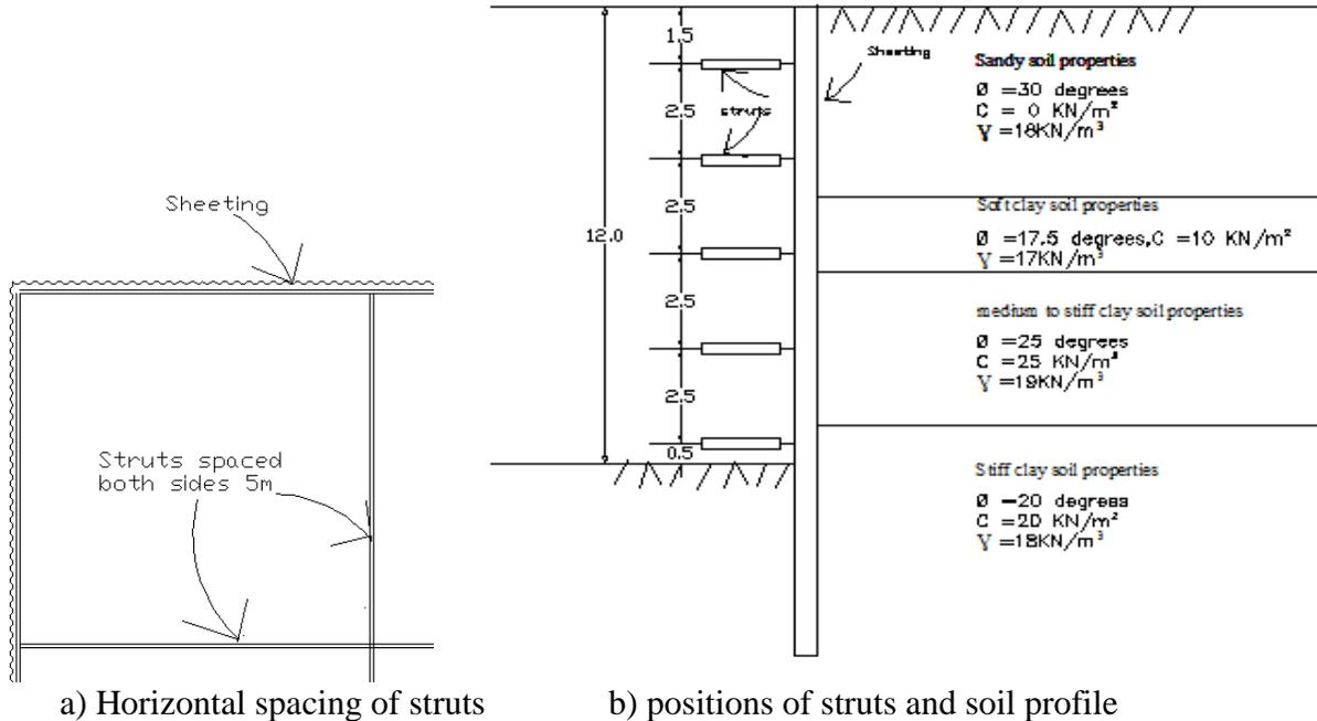
Figure 3-4: supporting system of braced excavation for stratified soil type 2
