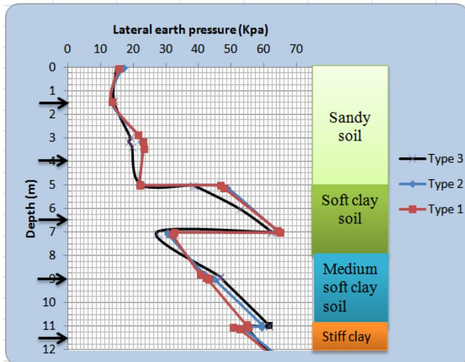
Figure 4-12: Lateral Earth pressure variation due to stiffness of sheet pile of stratified soil type 2
