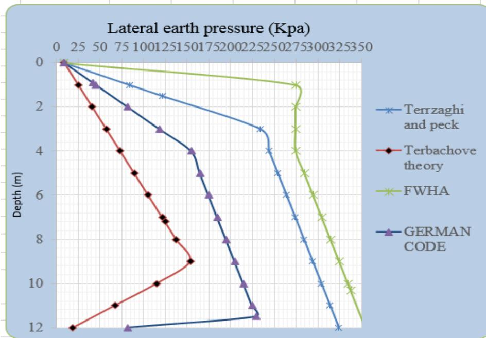
Figure 4-24: Apparent pressure using different approaches stratified soil type 2
