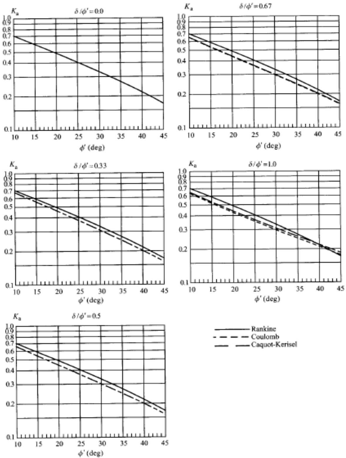
Figure 2-3 : coefficients of Rankin's, coulomb's and caquot-Kerisel's active earth pressure (horizontal component  $K_{a,h} = K_a \cos \delta$ )
