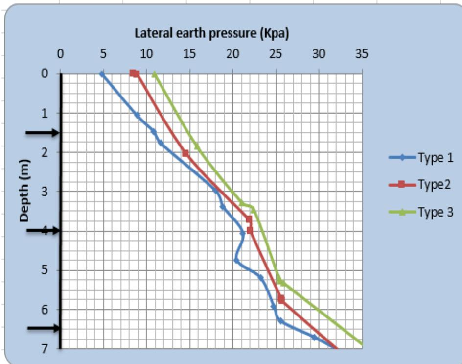
Figure 4-13: Lateral Earth pressure variation due to spacing of struts of sandy soil
