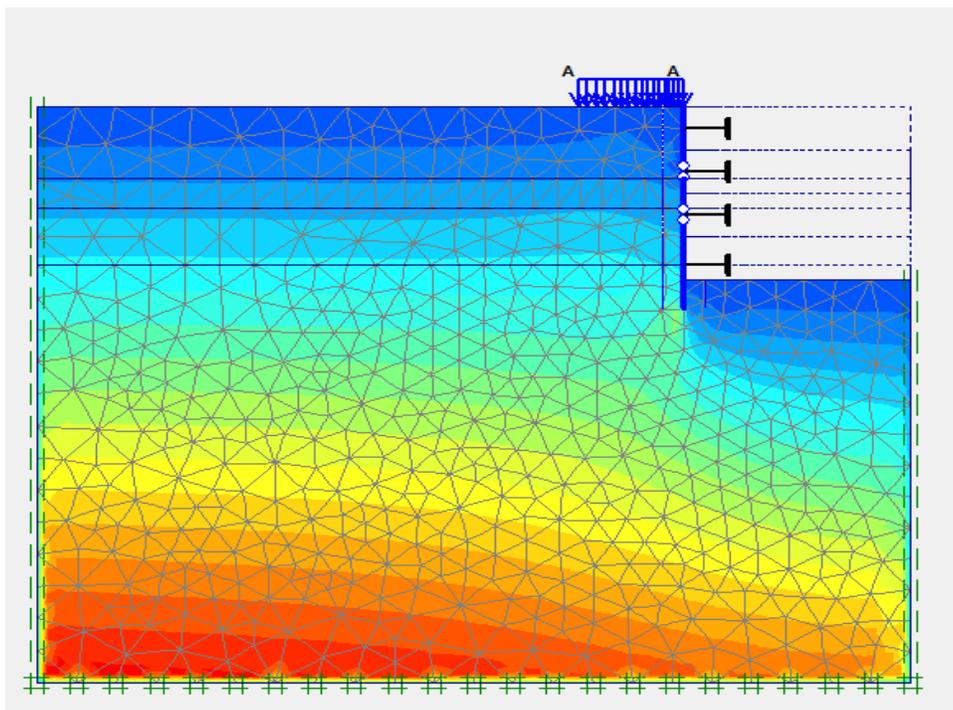
Figure A-5: Deformed shape of the geometry in stratified soil type 2
