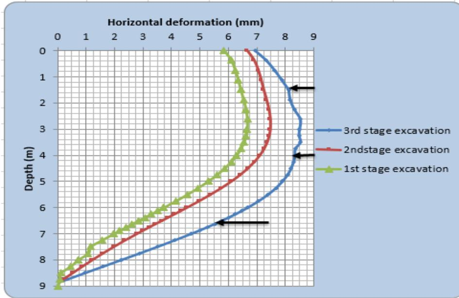
Figure A-8 Deformation of sheet piles at different stages of excavation of sandy soil
