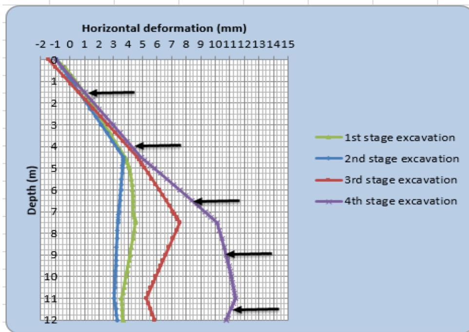
Figure A-11. Deformation of sheet piles at different stages of excavation stratified soil type 2
