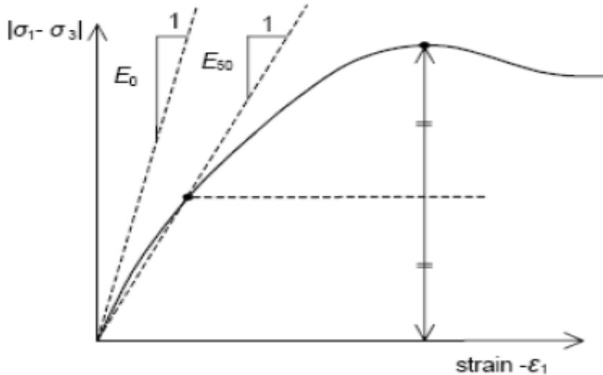
Figure A-7: Definition of  $E_0$  and  $E_{50}$  for standard drained triaxial test results
