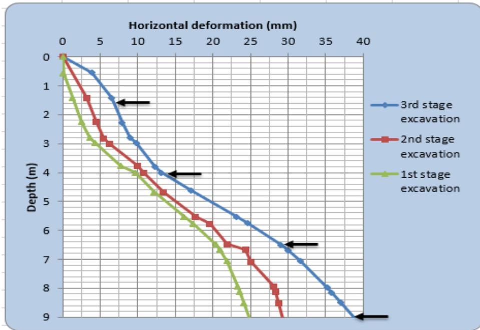
Figure A-10 Deformation of sheet piles at different stages of excavation stratified soil type 1
