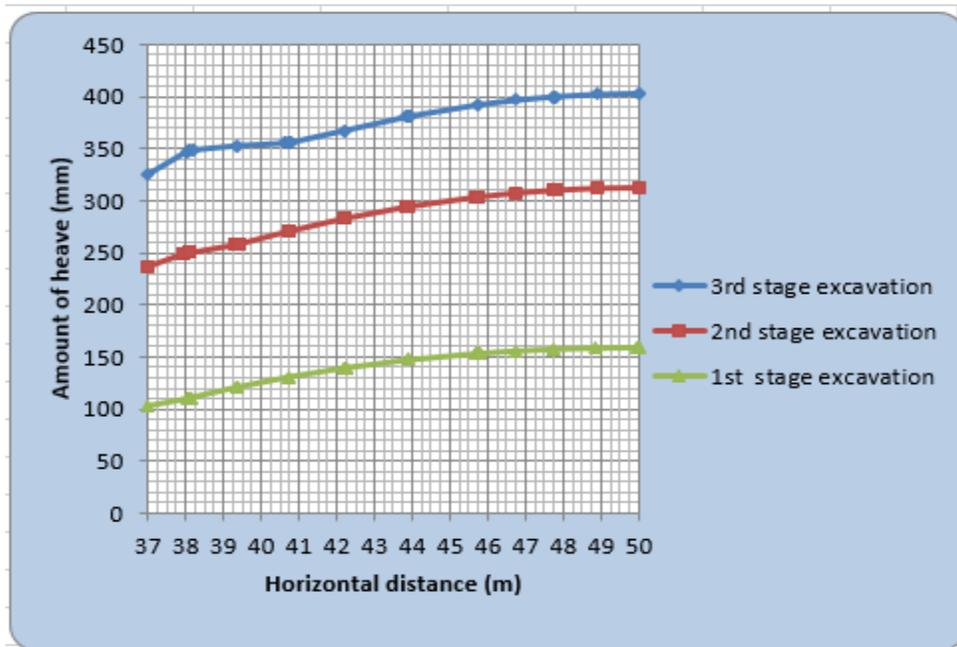
Figure A-21: Heave at bottom of excavation soft clay soil
