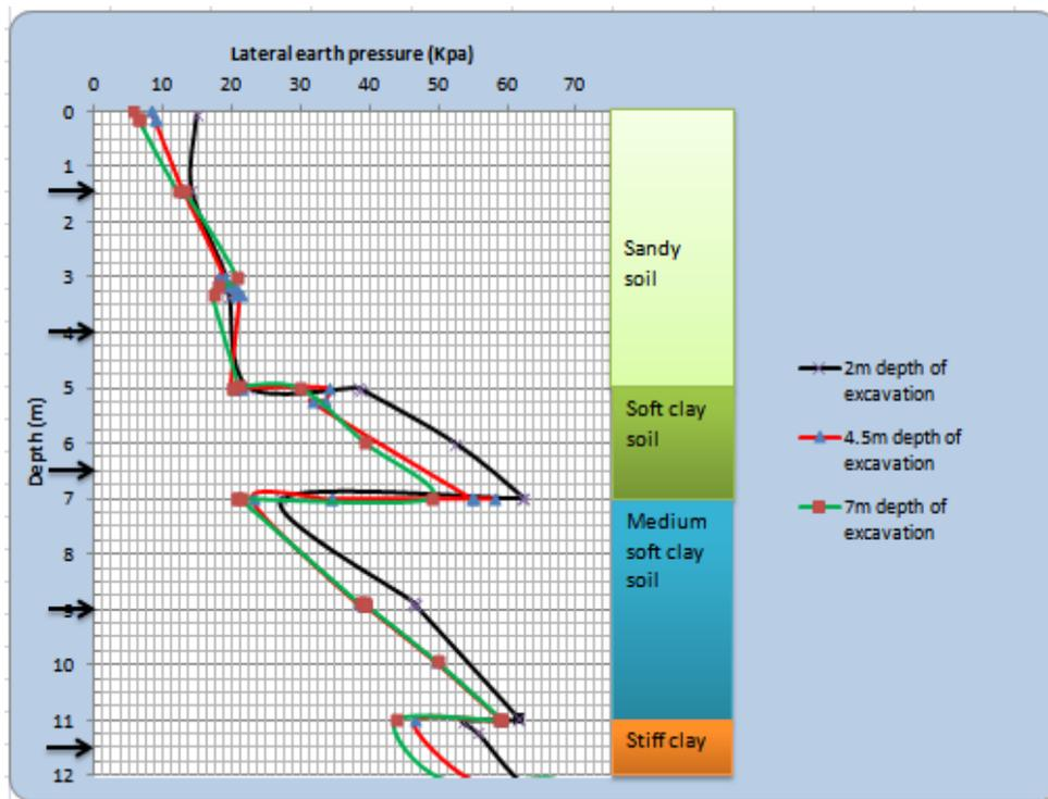
Figure 4-8: Lateral Earth pressure variation due to depth of embedment of stratified soil type 2
