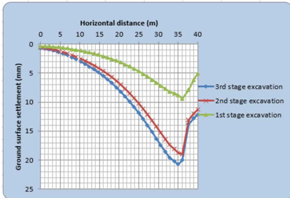
Figure A-16: Ground surface settlement of sandy soil
