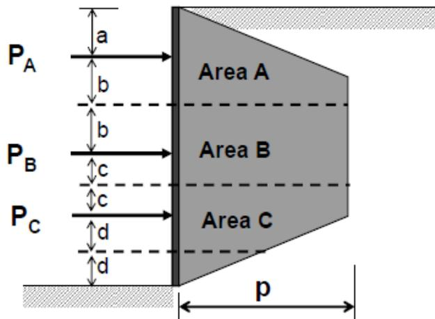
Figure 2-11: Calculation of struts using Tributary Area Method
