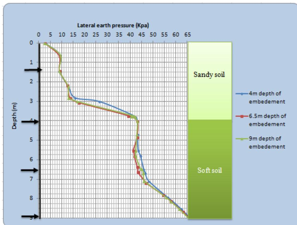
Figure 4-7: Lateral Earth pressure variation due to depth of embedment of stratified soil type 1
