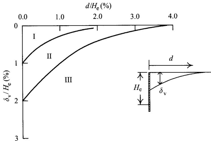
Figure 2-13: Peck's method (1969) for estimating ground surface settlement
