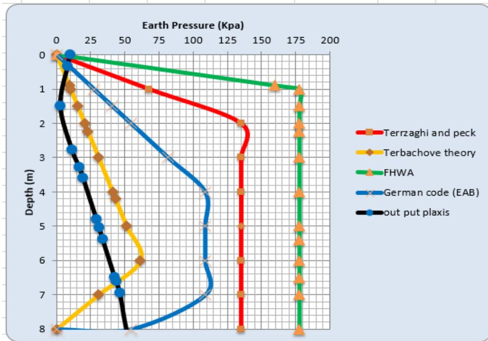
Figure 4-27: Comparison of different lateral earth pressure theories with Plaxis for soft clay soil
