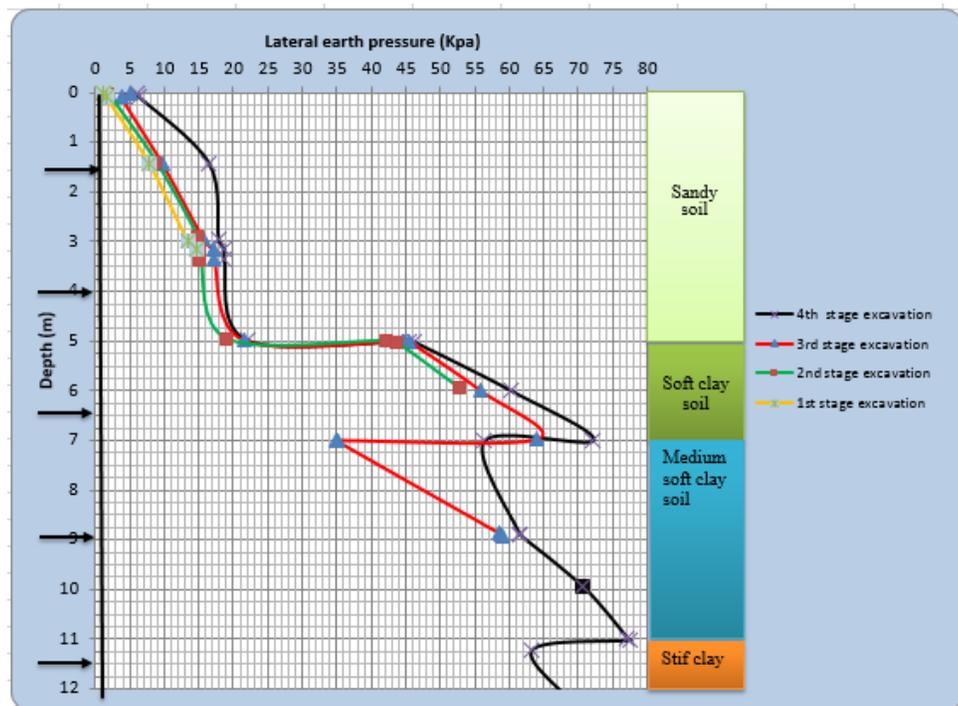
Figure 4-4: Lateral earth pressure at different stages of excavation for stratified soil type 2
