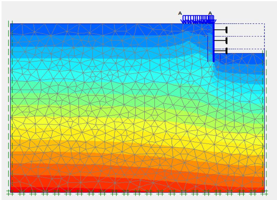
Figure A-2: Deformed shape of the geometry in sandy soil
