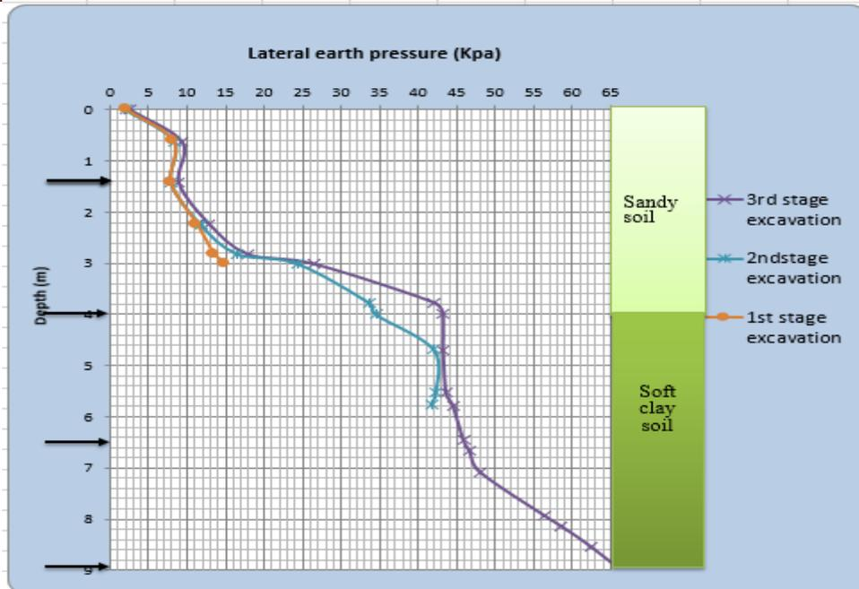
Figure 4-3 : Lateral earth pressure at different stages of excavation for stratified soil type 1
