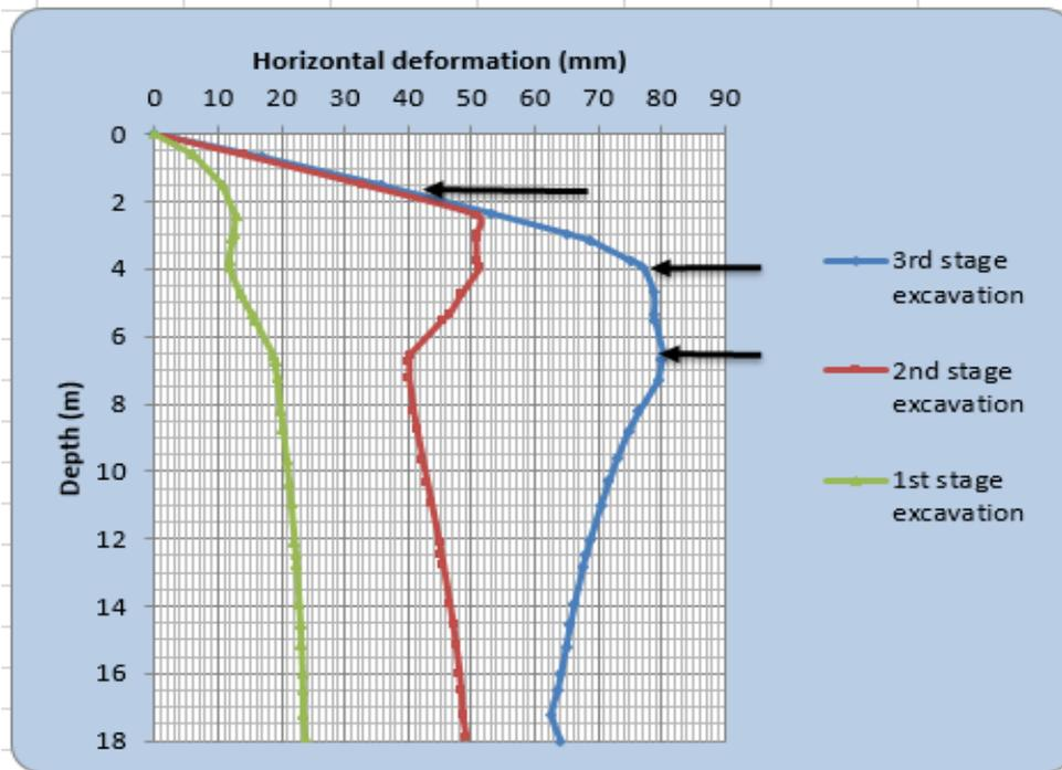
Figure A-9: Deformation of sheet piles at different stages of excavation soft clay soil
