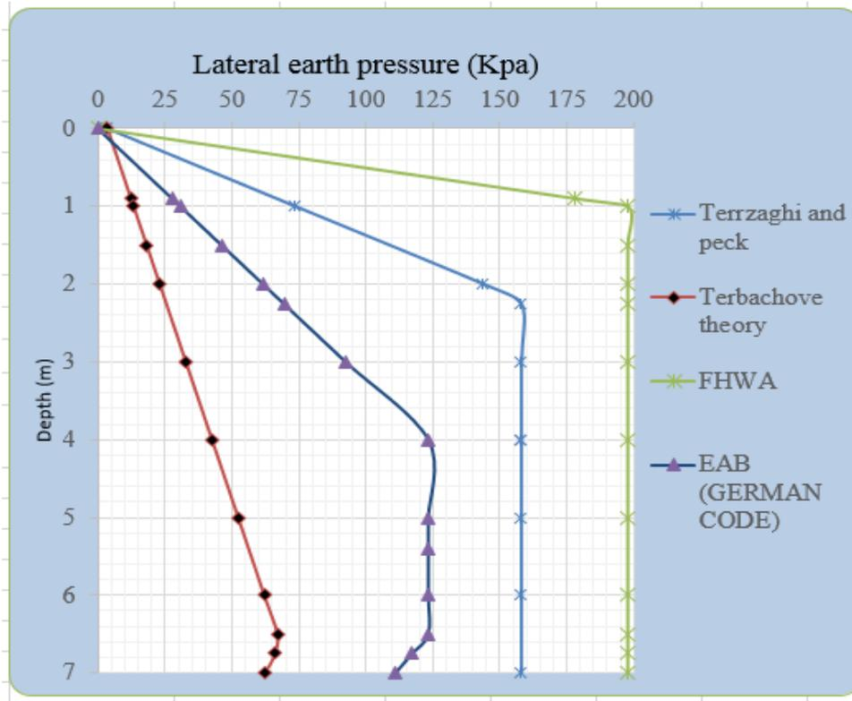
Figure 4-23: Apparent pressure using different approaches stratified soil type 1
