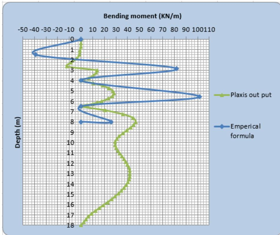
Figure 4-35: Bending moment for soft clay soil
