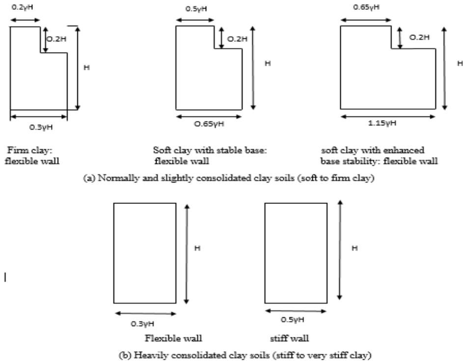
Figure 2-10: Earth pressure distribution on flexible and rigid walls for clay soils (Twine and Roscoe, 1999)
