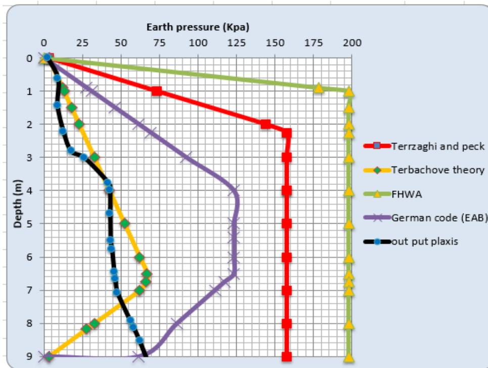
Figure 4-28 : Comparison of different lateral earth pressure theories with Plaxis for stratified soil type 1
