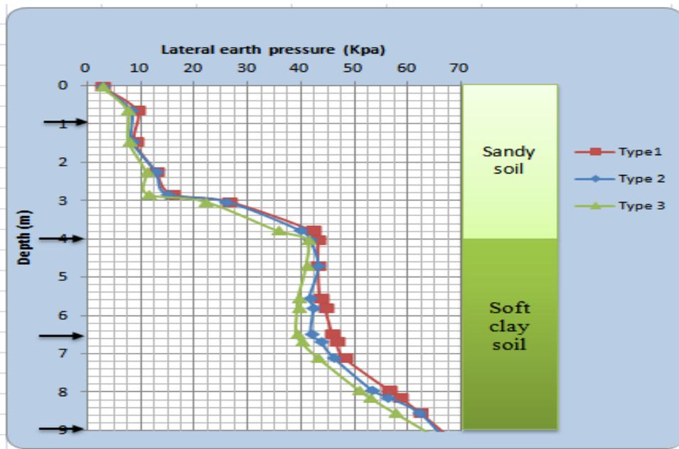
Figure 4-19: Lateral Earth pressure variation due to stiffness of struts of stratified soil type 1
