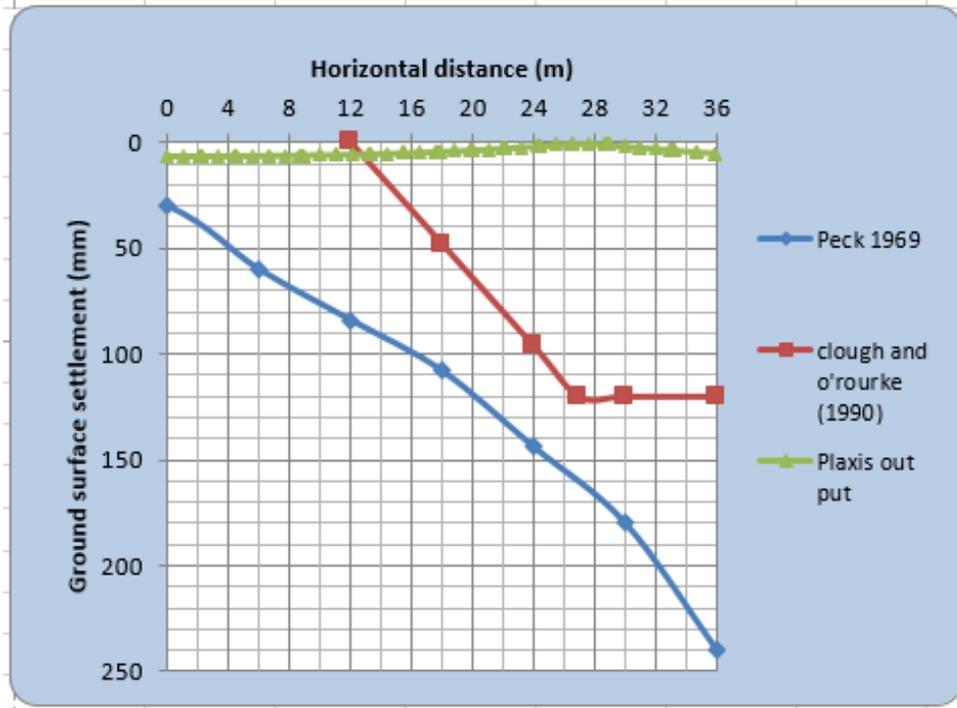
Figure 4-33: Ground surface settlement for stratified soil type 2
