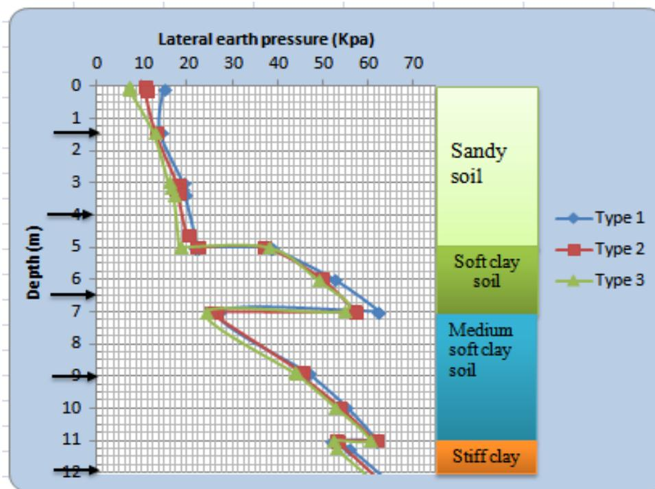
Figure 4-20: Lateral Earth pressure variation due to stiffness of struts of stratified soil type 2
