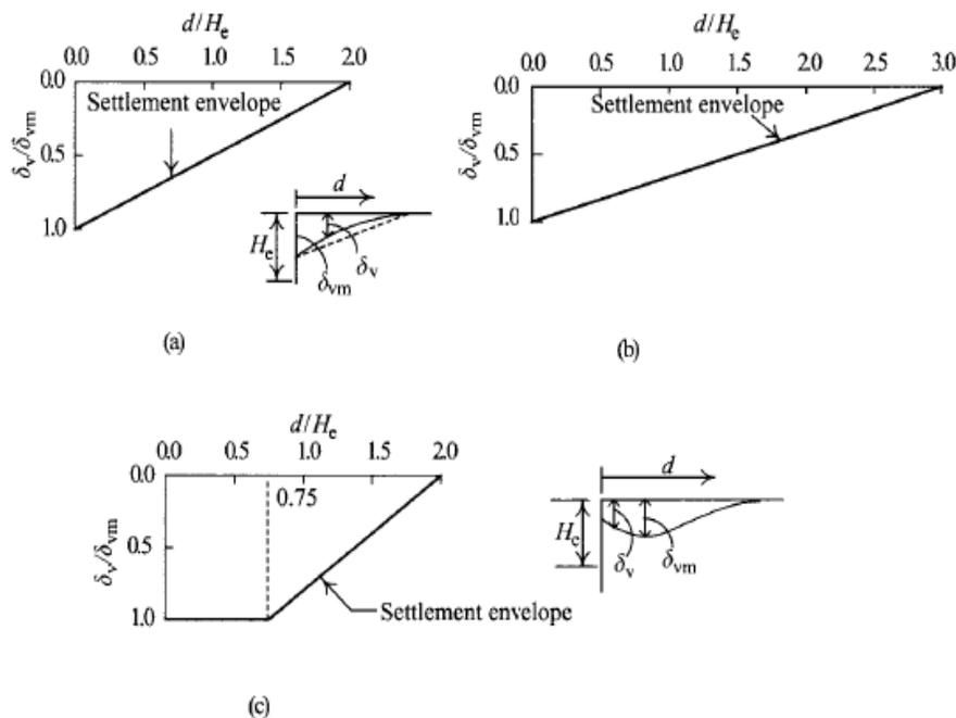
Figure 2-14: Method of Clough and O'Rourke (1990) for estimating ground surface settlement (a) Sand (b) Stiff to very stiff clay, and (c) soft to medium soft clay
