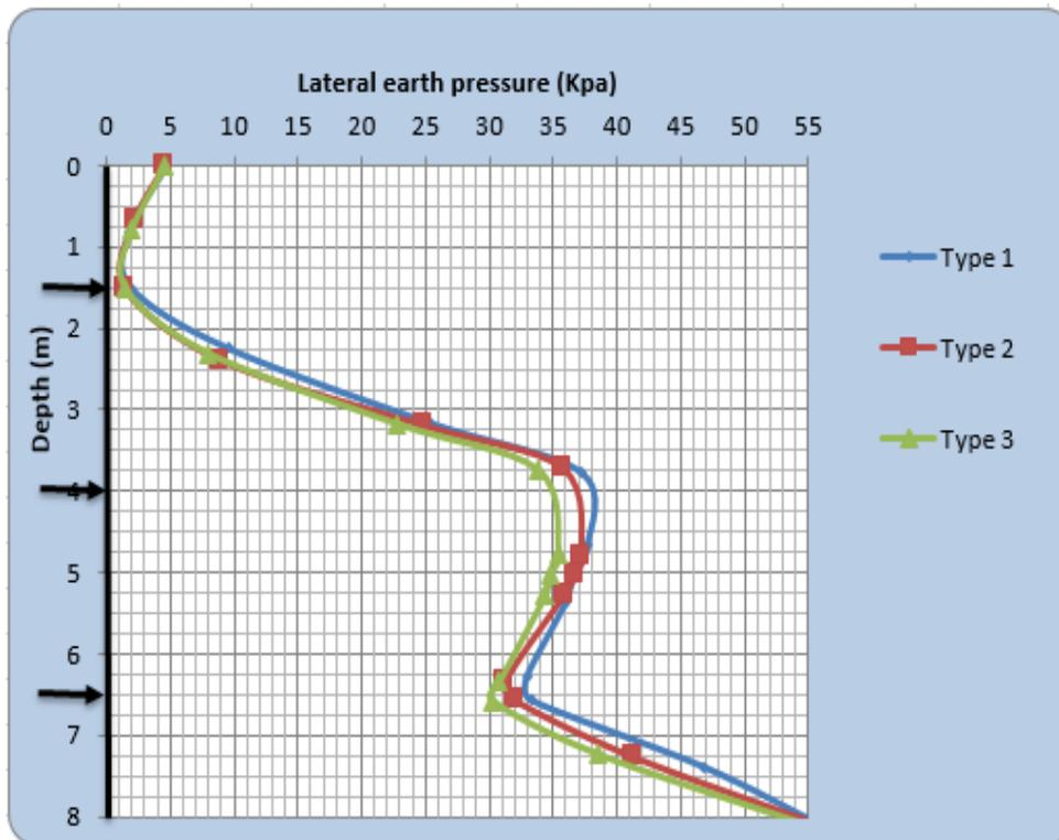
Figure 4-18: Lateral Earth pressure variation due to stiffness of struts of soft clay soil
