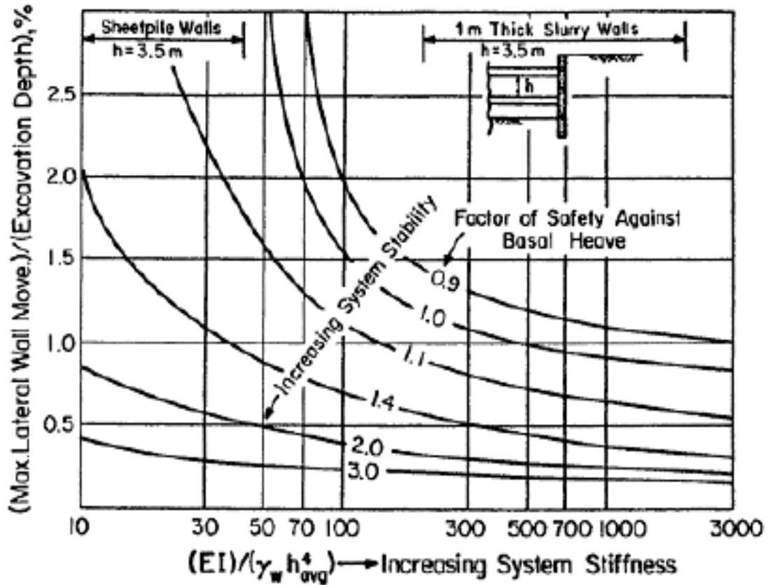
Figure 4-25: Correlation for Maximum Lateral Wall Deflection with Factor of safety Against Basal Heave and System Stiffness [Clough and O'Rourke, 1990]
