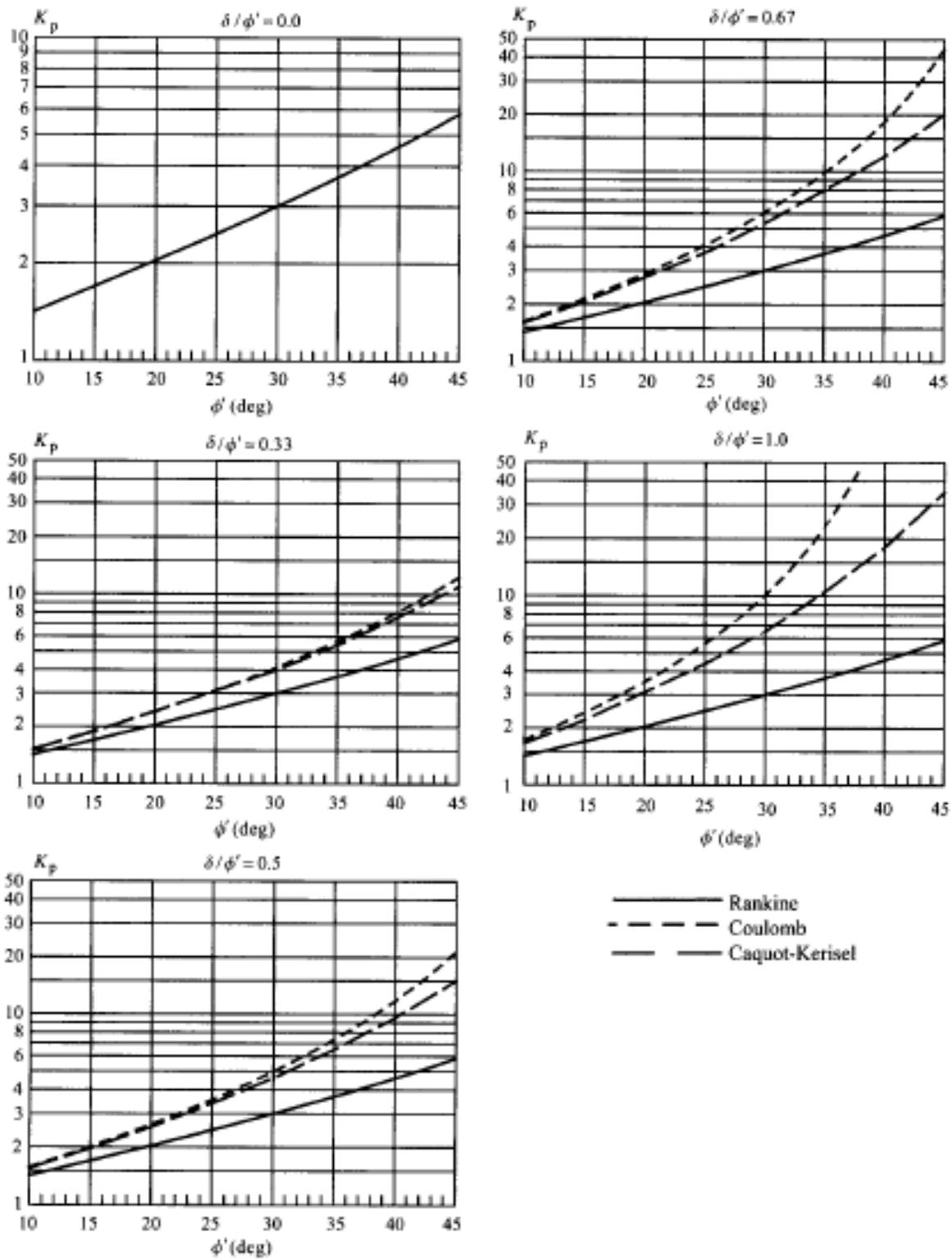
Figure 2-4: coefficients of Rankin's, coulomb's and caquot-Kerisel's passive earth pressure (horizontal component  $K_{p,h}=K_p \cos \delta$ )
