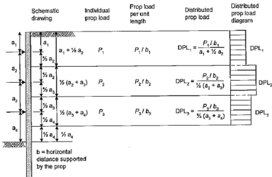
Figure 2-12: Example of Strut Force Calculation by DPL Method using Tributary Area Method
