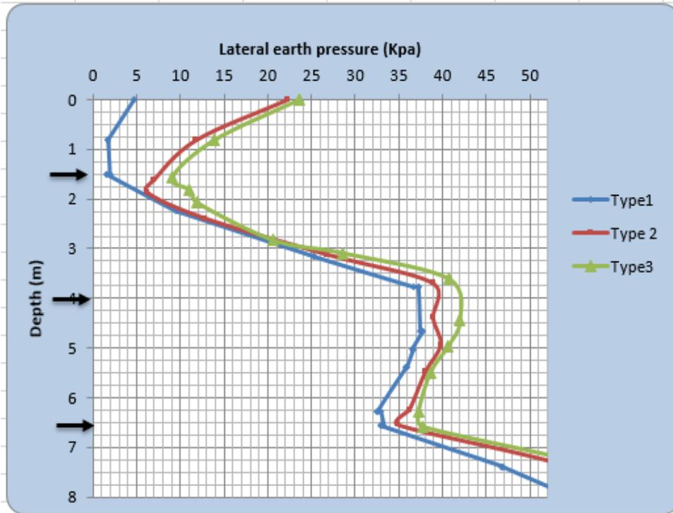
Figure 4-14: Lateral Earth pressure variation due to spacing of struts of soft clay soil
