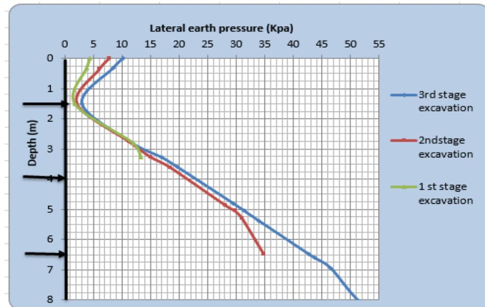
Figure 4-2: Lateral earth pressure at different stages of excavation soft clay soil
