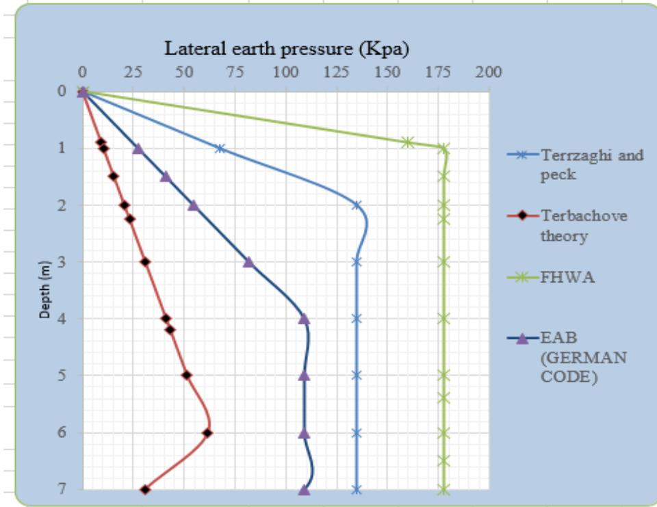
Figure 4-22: Apparent pressure using different approaches soft clay soil
