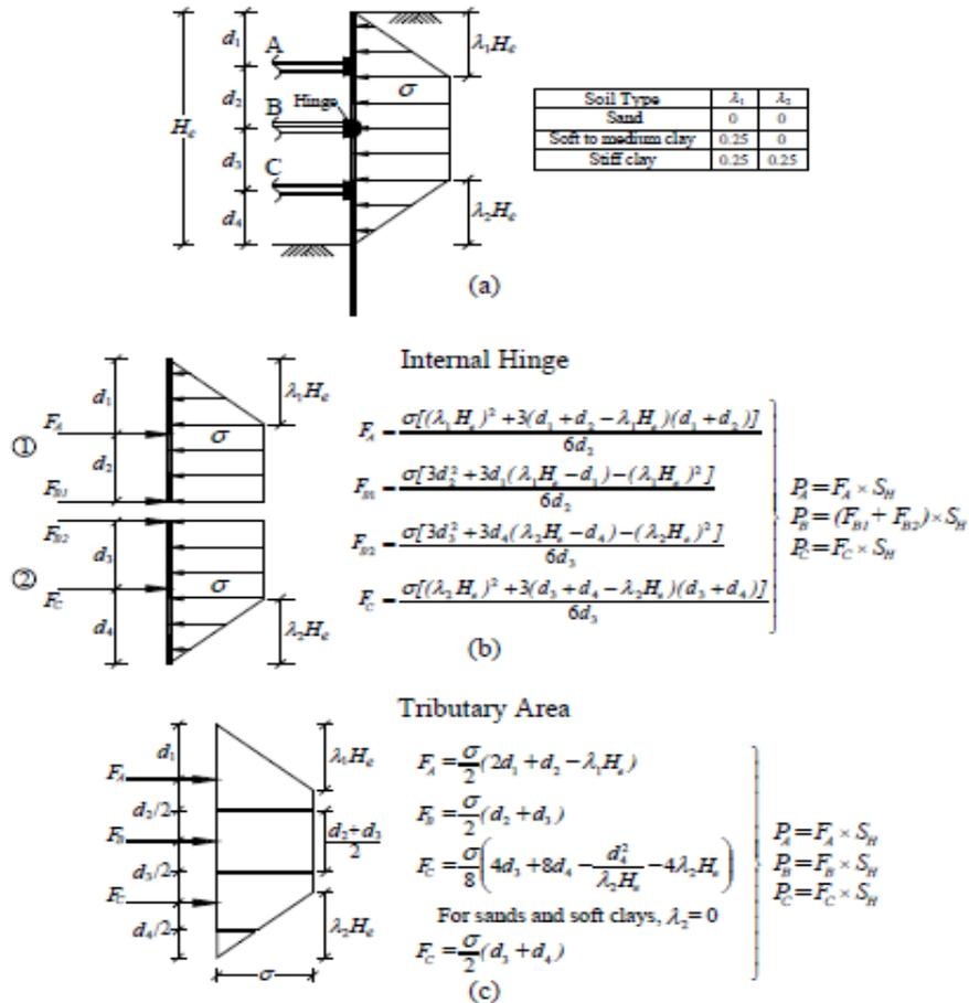
Figure A-1: calculation of strut loads
