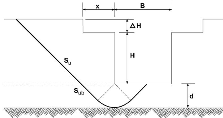
Figure 2-9: Henkel's mechanism of base failure.
