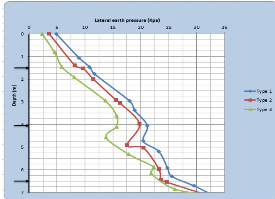
Figure 4-17: Lateral Earth pressure variation due to stiffness of struts of sandy soil
