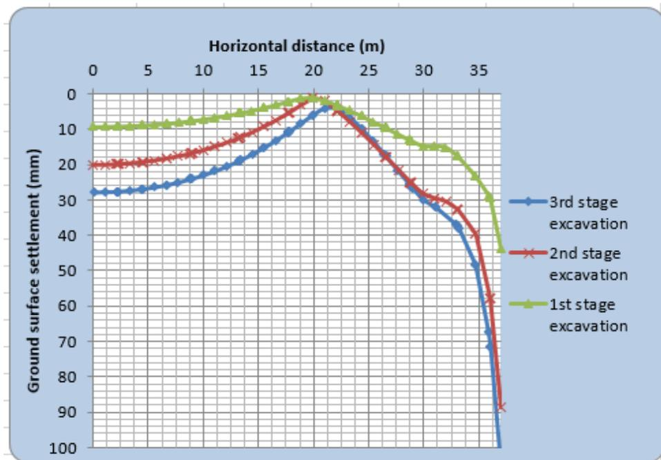
Figure A-17: Ground surface settlement softy clay soil
