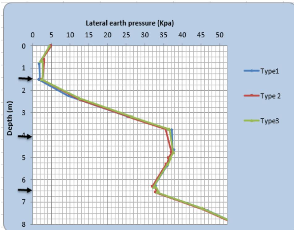
Figure 4-10: Lateral Earth pressure variation due to stiffness of sheet pile of soft clay soil
