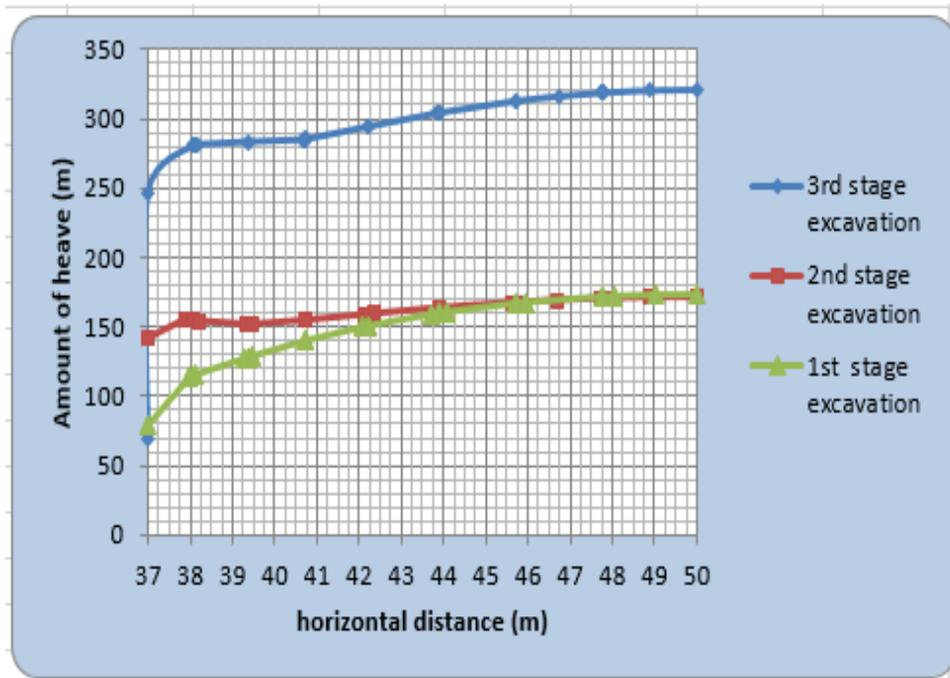
Figure A-22: Heave at bottom of excavation stratified soil type 1
