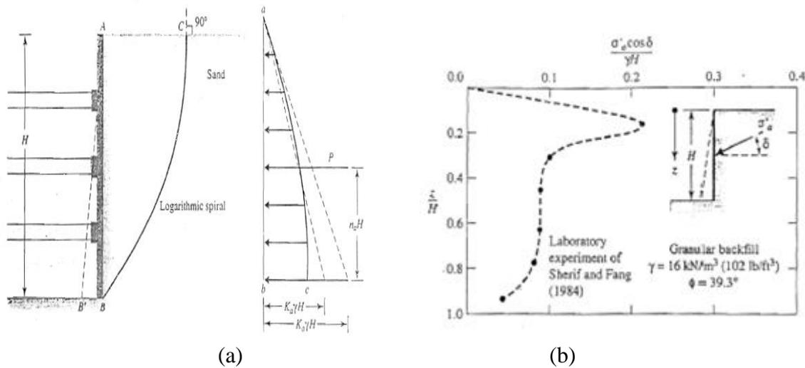
Figure 2-5: (a) Earth pressure in braced Excavation (Das, 1999): (b) Field Measurement of Earth Pressure in Braced Excavation (Sheriff and Fang, 1984)
