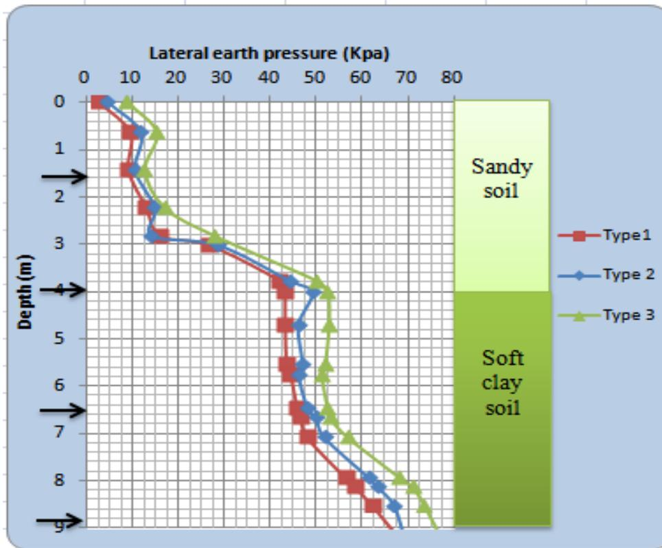
Figure 4-15: Lateral Earth pressure variation due to spacing of struts of stratified soil type 1
