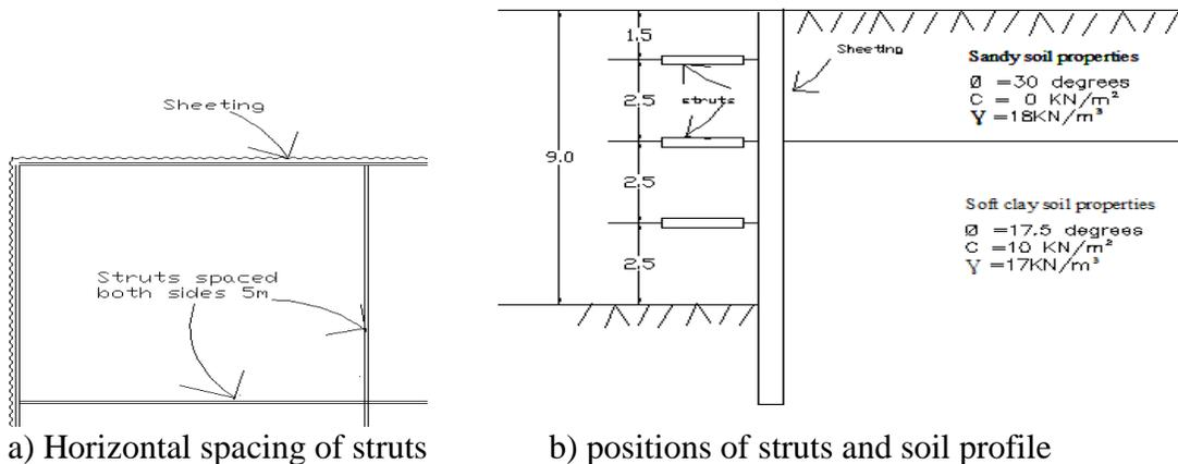
Figure 3-3: supporting system of braced excavation for stratified soil type 1
