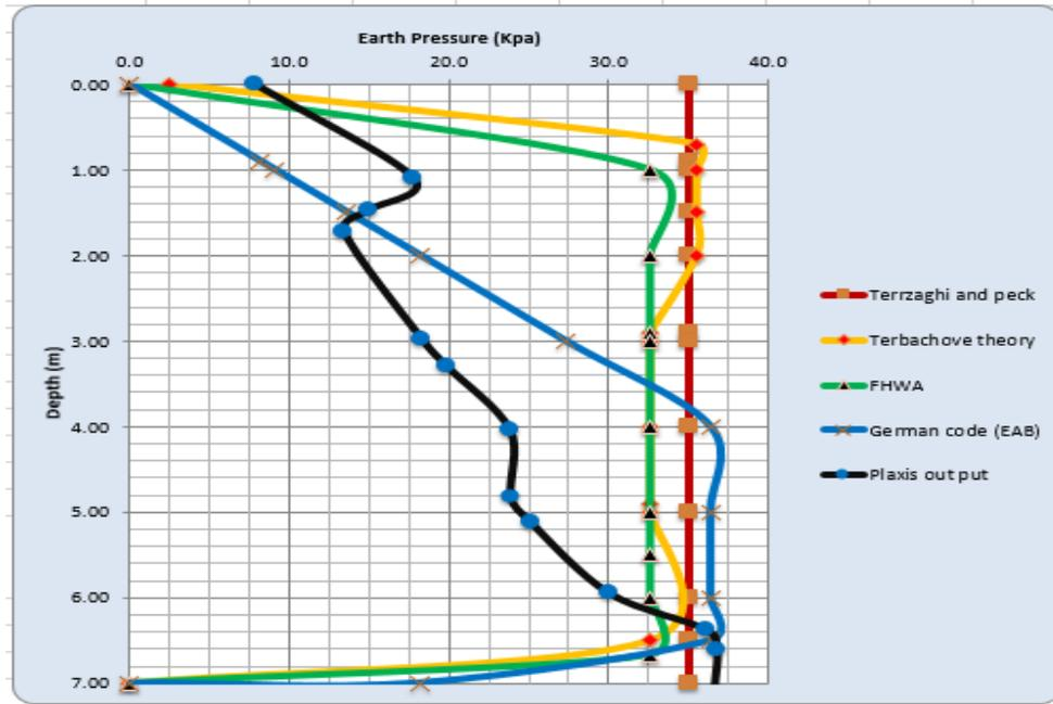
Figure 4-26: Comparison of different lateral earth pressure theories with Plaxis for sandy soil
