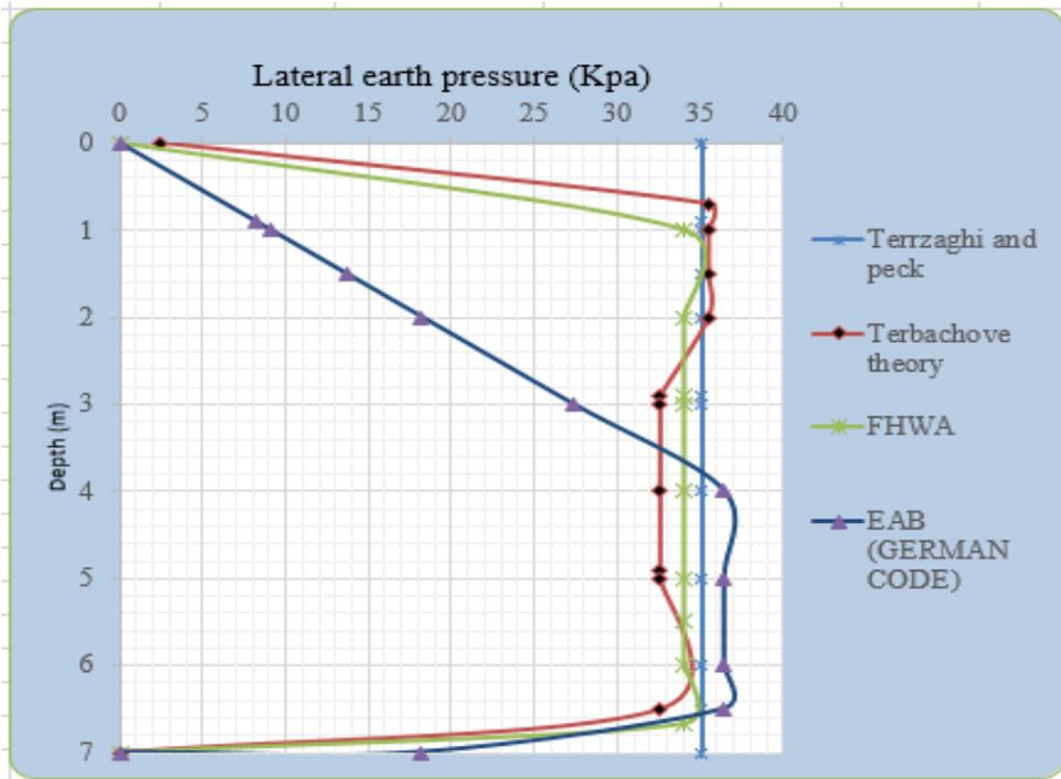
Figure 4-21: Apparent pressure using different approaches sandy soil
