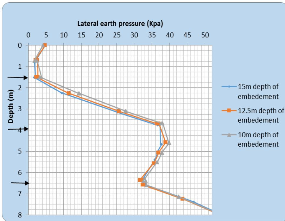
Figure 4-6: Lateral Earth pressure variation due to depth of embedment of soft clay soil
