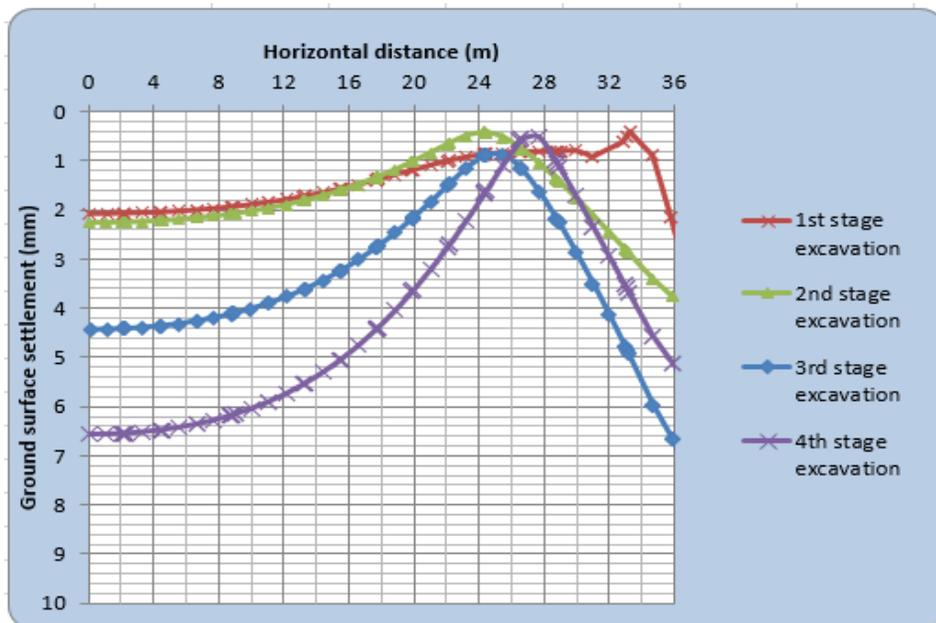
Figure A-19: Ground surface settlement stratified soil type 2
