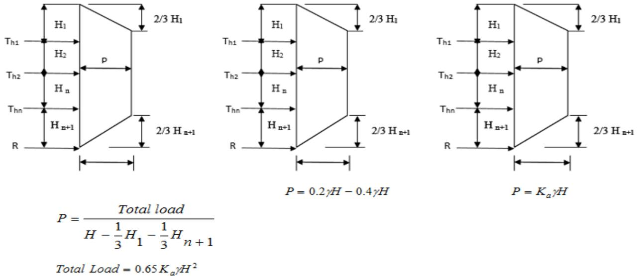
Figure 2-8 (a): Apparent pressure diagram for sand
