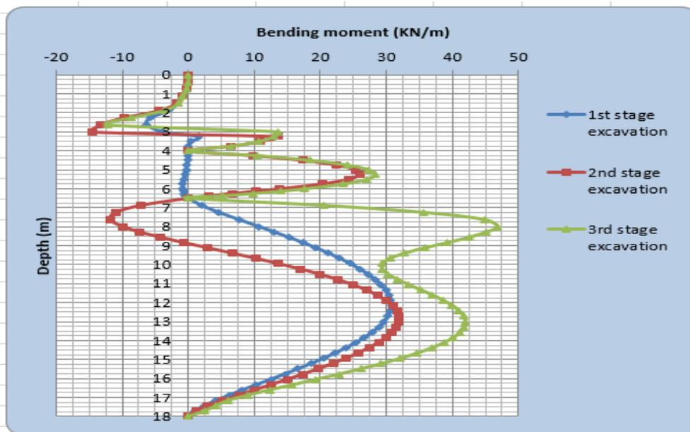
Figure A-13: Bending moment of the sheet pile wall at stages of excavation soft clay soil
