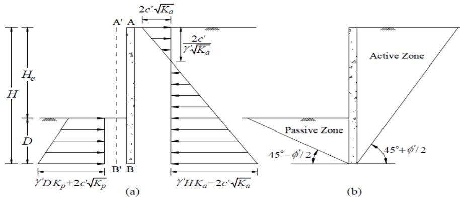
Figure 2-1 : (a) Rankine's pressure distributions, and (b) Passive and Active Zones
