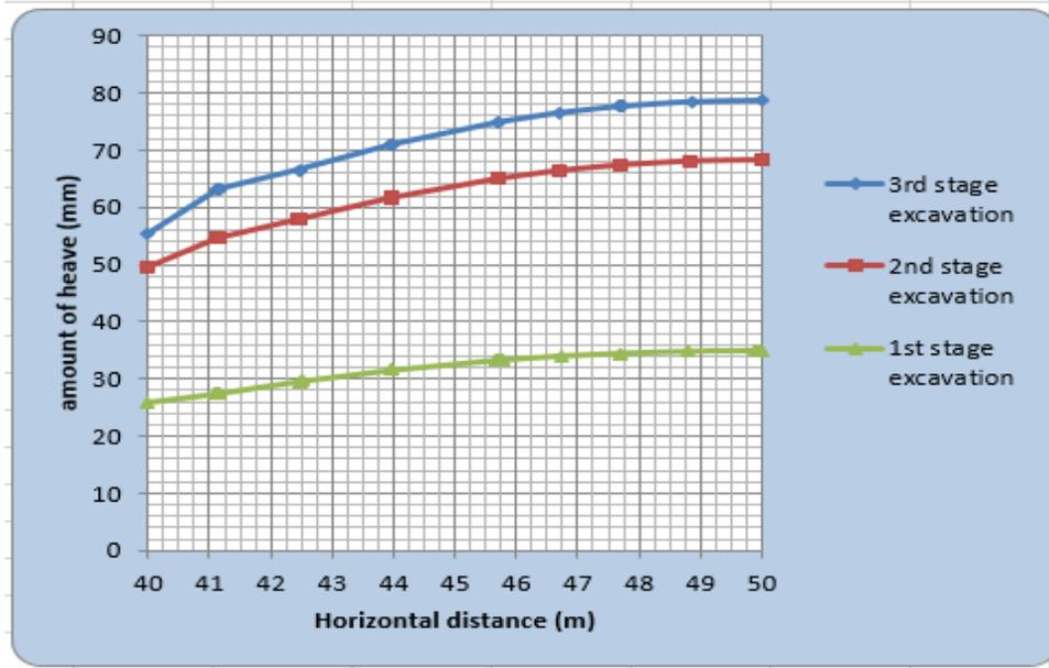
Figure A-20: Heave at bottom of excavation sandy soil
