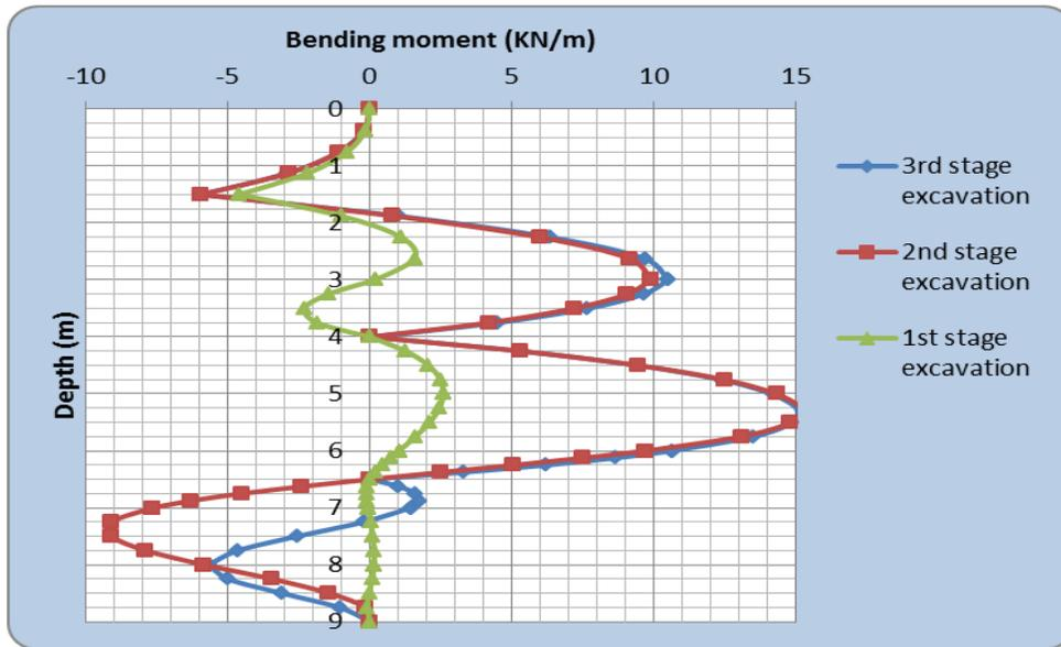
Figure A-12: Bending moment of the sheet pile wall at stages of excavation of sandy soil
