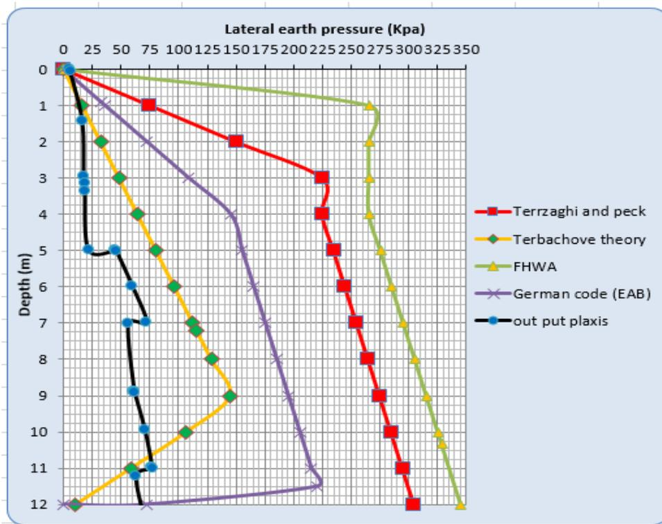
Figure 4-29 : Comparison of different lateral earth pressure theories with Plaxis for stratified soil type 2
