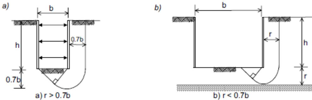
Figure 2-16: Bottom heave analysis for deep excavations ( $h/b < 1$ ) (after Terrzaghi 1943)
