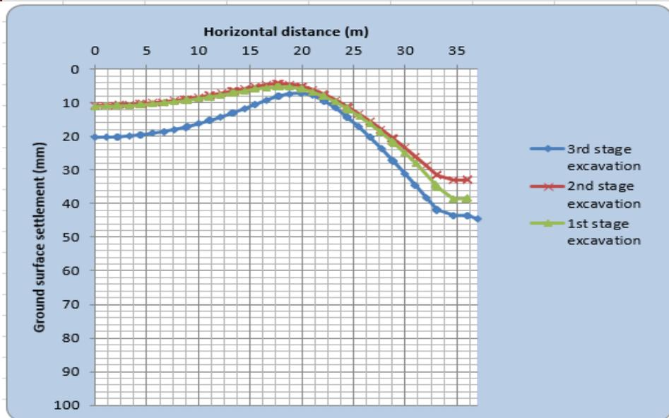
Figure A-18: Ground surface settlement stratified soil type 1
