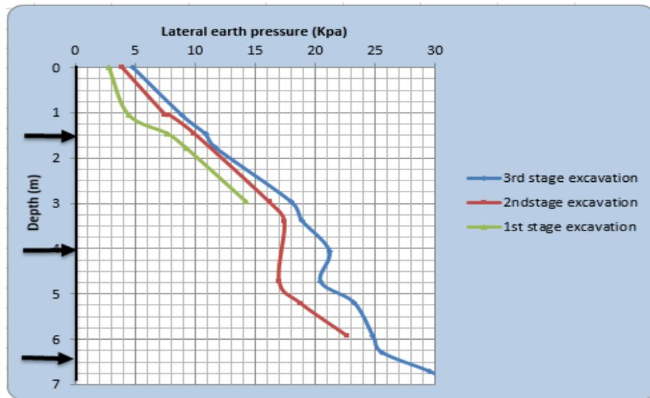
Figure 4-1: Lateral earth pressure at different stages of excavation for sandy soil
