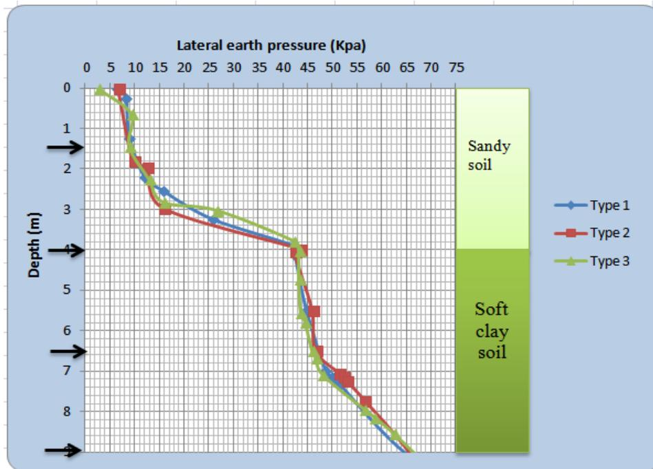
Figure 4-11: Lateral Earth pressure variation due to stiffness of sheet pile of stratified soil type 1
