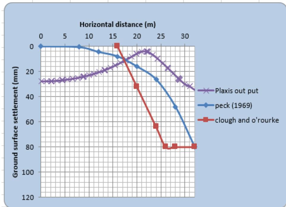
Figure 4-31: Ground surface settlement for soft clay soil
