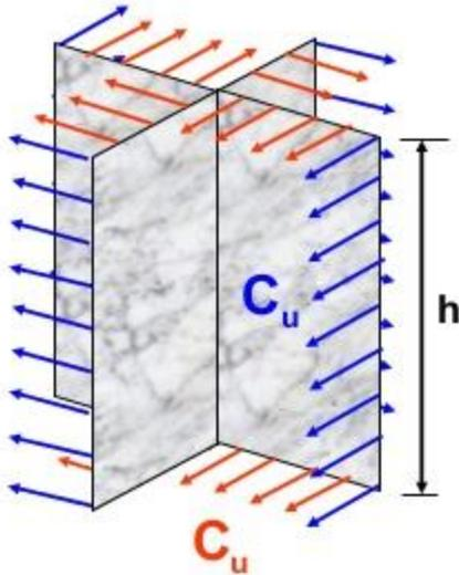
Since the test is very fast, Unconsolidated Undrained (UU) can be expected
