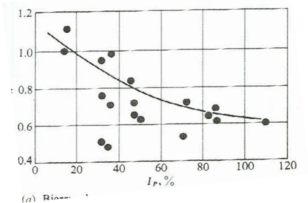
Figure 1.8: Bjerrum's correction factor for vane shear test.
