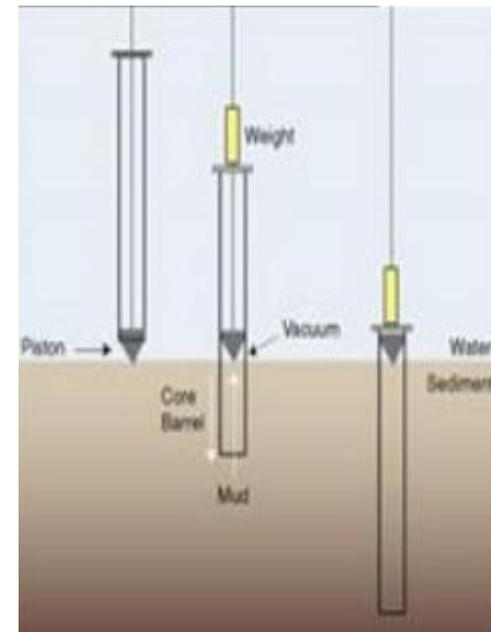
Provides the best undisturbed samples of cohesive soils.
