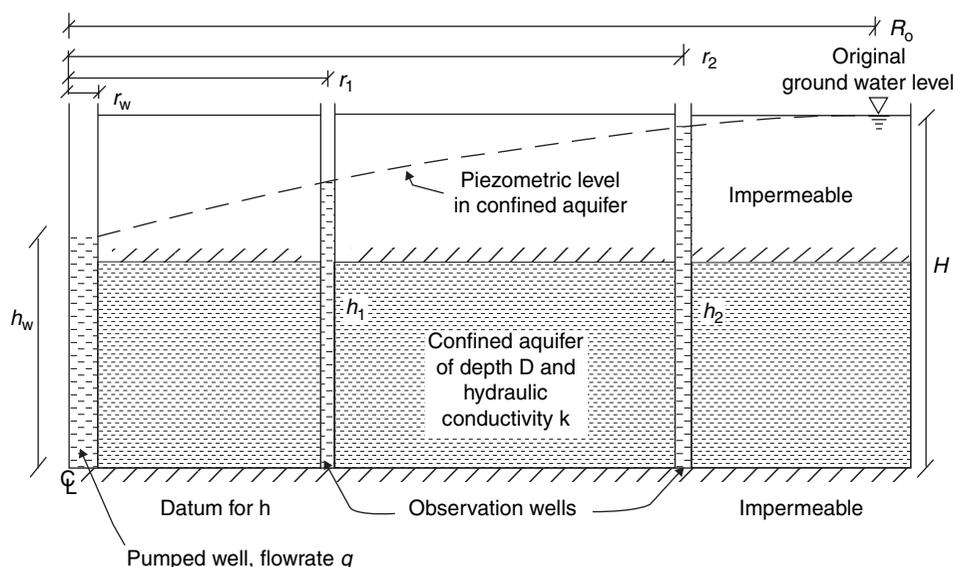
**Figure 16.2** Radial flow to a fully penetrating well in a confined aquifer
