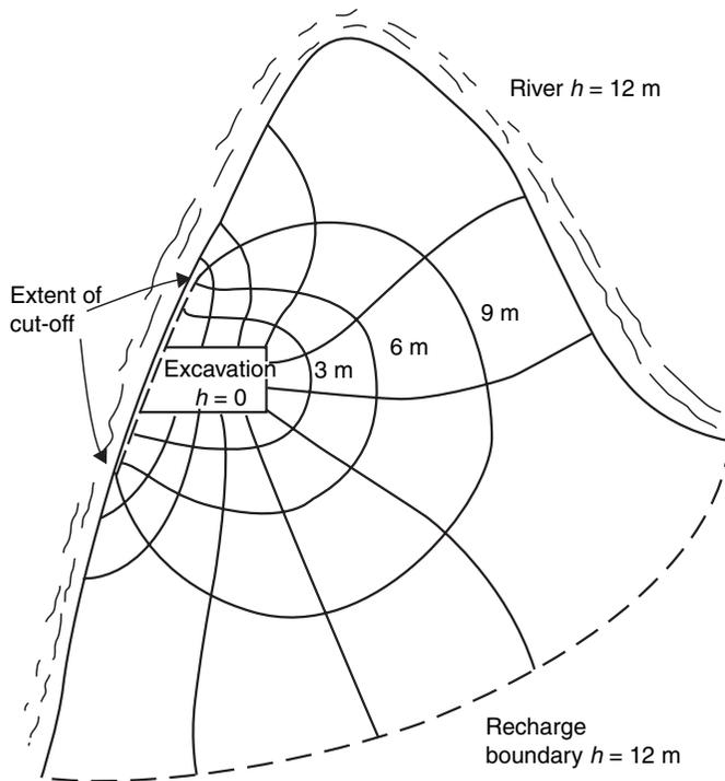
**Figure 16.5** Example of a horizontal plane flownet, for flow to an excavation in a deep chalk aquifer on the Medway peninsula
