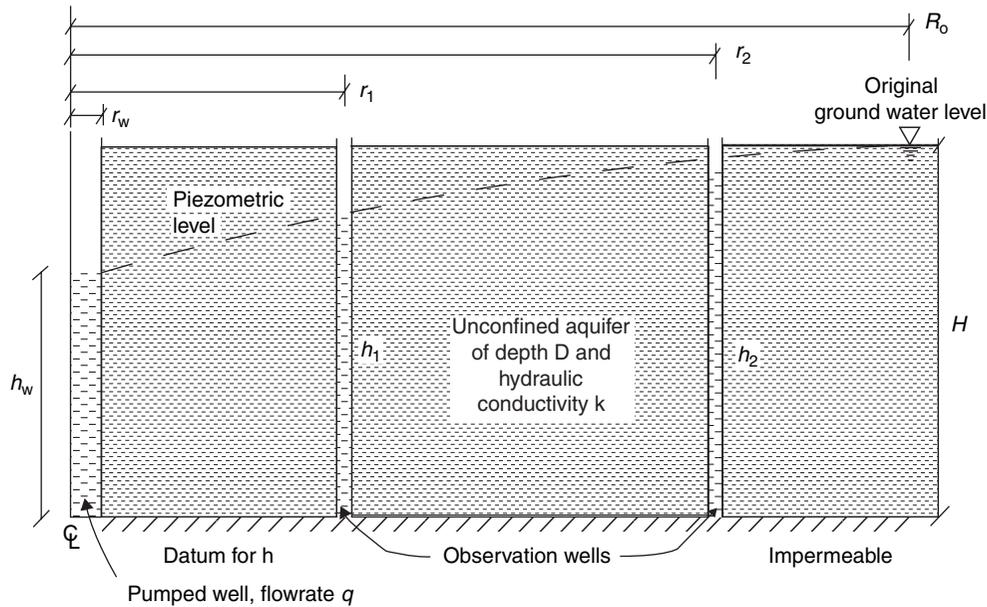
**Figure 16.3** Radial flow to a fully penetrating well in an unconfined aquifer
