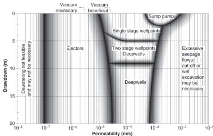
**Figure 16.7** Range of application of dewatering techniques
