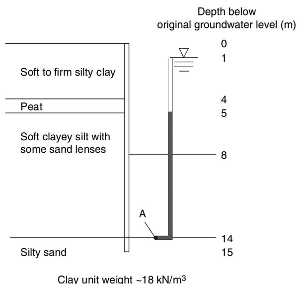
**Figure 16.6** Case study demonstrating the importance of controlling pore water pressures to an adequate depth below the excavation floor
