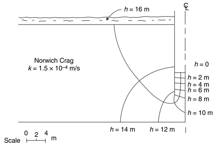
**Figure 16.4** Example of a plane flownet in one half of the vertical cross-sectional plane for flow into a trench excavation
