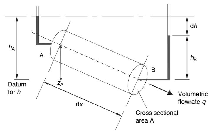
**Figure 16.1** Schematic representation of hydraulic gradient and Darcy's Law
