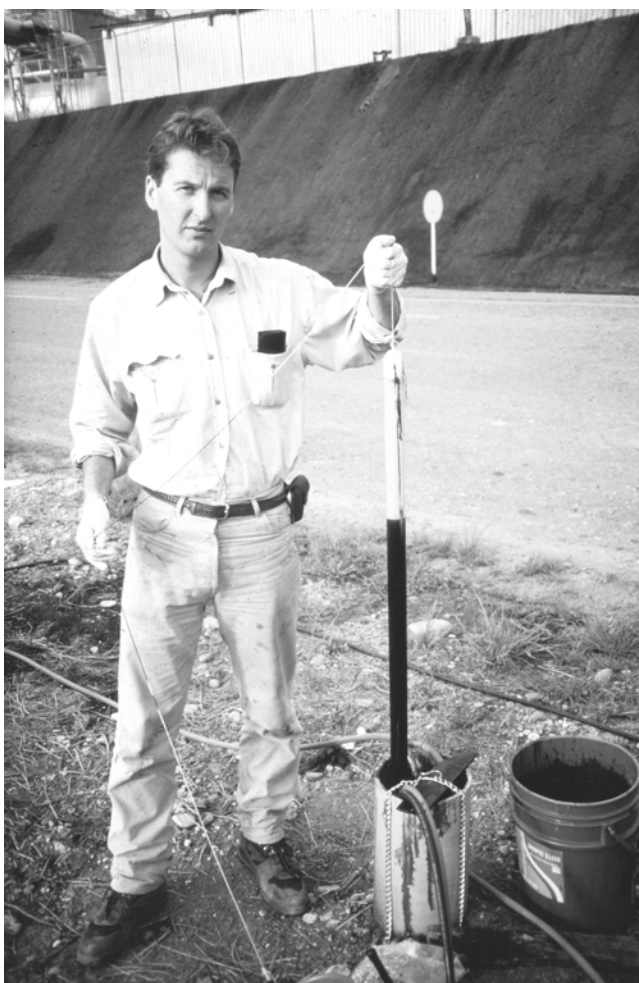
FIGURE 3.18 One of the authors holding a bailer containing LNAPL recovered from the groundwater surface at the site.
