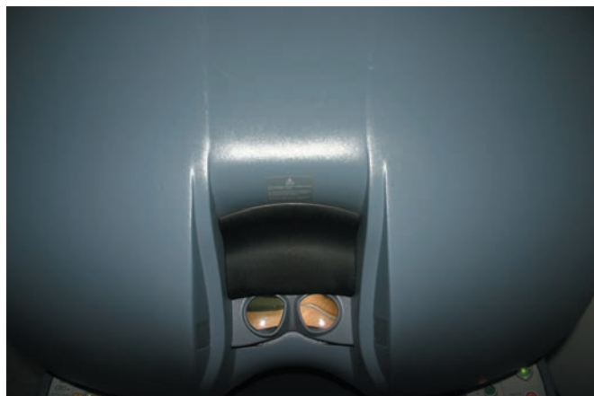
Figure 7.4 da Vinci console, binocular viewer (photo courtesy of Daniel Leff).
