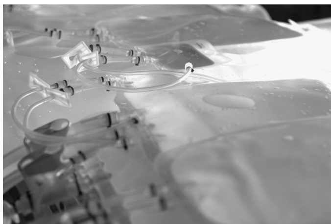
Figure 9.3 Continuous biomanufacturing capable Thermo TM Scientific TM BioProcess Container assembly.
