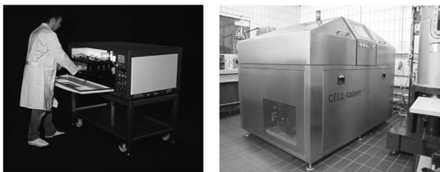
Figure 7.5 CELL-tainer ® single-use bioreactor at 20 and 200 l scale.
