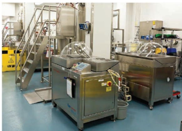
Figure 18.2 Continuous centrifugation units used for a perfusion process (from Ref. [18]). Copyright 2012 held by Shire with all rights reserved. No party may make any use of this image without the express written permission of Shire.
