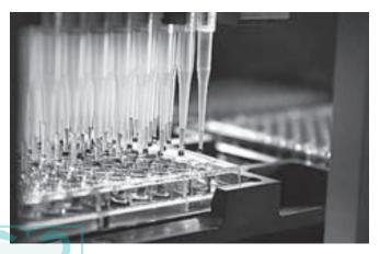
FIGURE 7.1 A pipetting robot system for fully automated high-throughput screening arrays.
