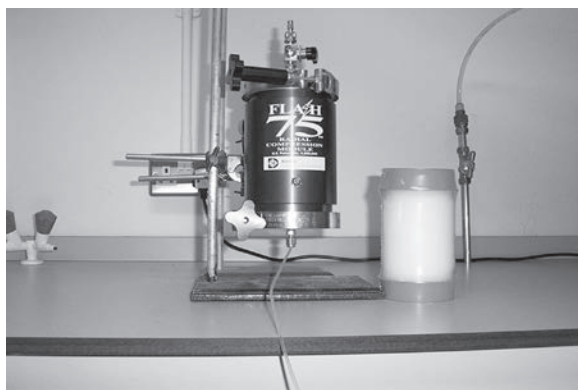
Fig. 8.4 Biotage™ flash chromatograph. Fast separations are achieved with good resolution.
