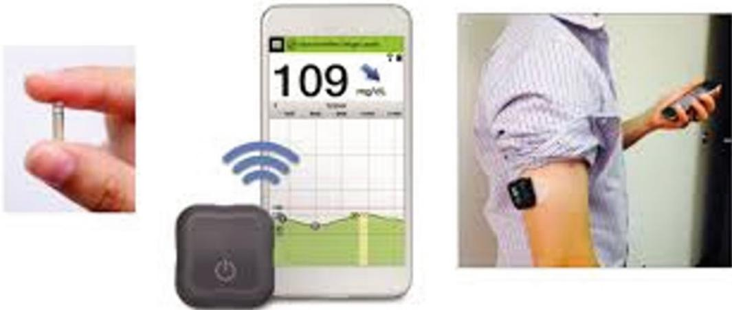
**Fig. 6** Long-term glucose sensor with transmitter and smartphone control (Senseonic)
