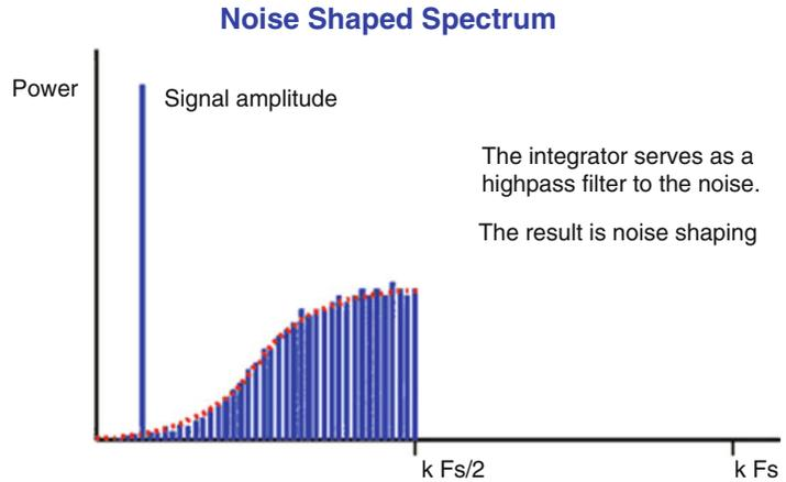
**Fig. 6** Effect of the digital filter on the shaped noise
