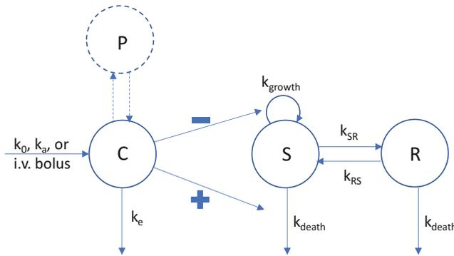
**Fig. 5** Schematic illustration of the pharmacokinetic/pharmacodynamic model. *C* central compartment; *P* peripheral compartment; *S* proliferating and drug-sensitive bacteria; *R* resting and drug-insensitive bacteria;  $k_0$  drug infusion rate constant;  $k_a$  drug absorption rate constant;  $k_e$  drug elimination rate constant;  $k_{\text{growth}}$  and  $k_{\text{death}}$  rate
