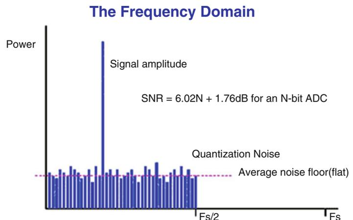
By splitting the fundamental amplitude by the RMS sum of all the frequencies representing noise, we get the signal-to-noise ratio (SNR). For an  $N$ -bit ADC,  $SNR = 6.02 N + 1.76$  dB. To improve the SNR in a conventional ADC (and consequently the accuracy of signal reproduction), one must rise the number of bits.
