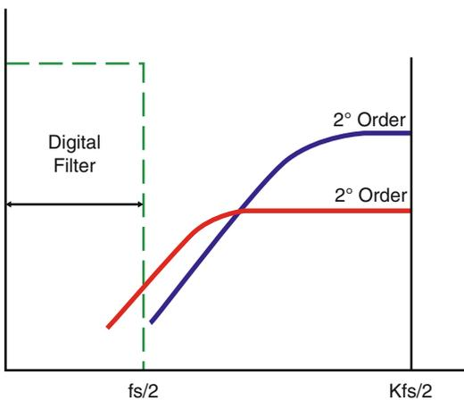
**Fig. 7** Using more than one integrator and summing stage to achieve a higher order of quantization noise
