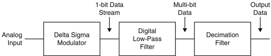
**Fig. 9** Digital side of sigma-delta modulator
