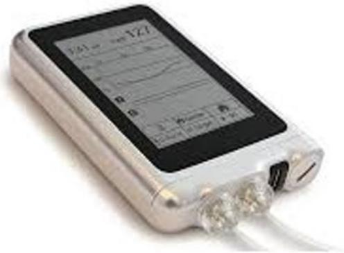
**Fig. 8** Bihormonal pump with two separate syringes for dispensing insulin and glucagon. Controlled by a CSGM sensor, data are transmitted to the pump and processed by an algorithm to keep glucose concentration within a predetermined range. Glucagon is dispensed when impending hypoglycemia is recognized by the algorithm
