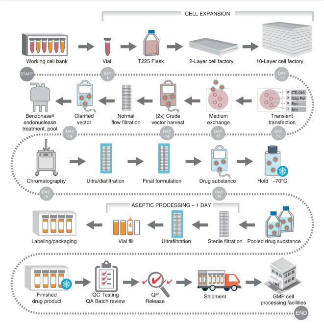
**Figure 17.20** Schematic overview of a lentiviral vector manufacturing process. The produced viral vector is used as starting material for the genetic modification of T-cells in the manufacture of a CAR-T product, reprinted with permission (Levine et al. 2017). A similar production approach is taken for other *ex-vivo* gene therapy as well as *in-vivo* gene therapy products (cf. Chap. 16). QC=quality control, QP=qualified person, QA=quality assurance
