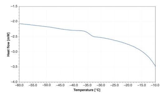
Figure 5.9 ■ Differential Scanning Calorimetry trace of a 5% sucrose solution with a Tg about -35 °C
