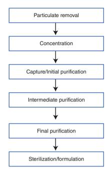
**Figure 4.3** Basic operations required for the purification of a biopharmaceutical macromolecule. For monoclonal antibody processes the concentration occurs within the capture step. Final purification is often called "polishing"
