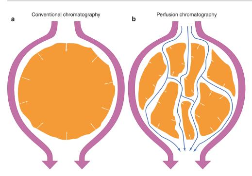
Figure 4.5 ■ The structure of conventional chromatographic particles (a) and the perfusion of flow through chromatographic particles (b) (adapted from Fulton 1994)
