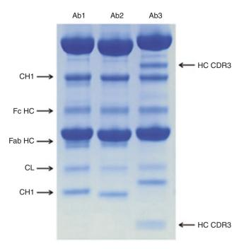
**Figure 3.8** ■ Fragmentation of three (Ab1, Ab2 and Ab3) monoclonal antibodies monitored using SDS-PAGE (*taken from Vlasak et al., MAbs (2011) 3:3, 253–263*); CH1—heavy chain constant domain 1, Fc HC—heavy chain Fc domain, Fab HC—heavy chain Fab domain, CL—light chain constant domain, HC—heavy chain, CDR3—complementarity-determining region 3
