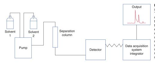
Figure 3.1 Components of a typical chromatography station. The pump combines solvents one and two in appropriate ratios to generate a pH, salt concentration, and/or hydrophobic gradient. Proteins that are fractioned on the column pass through a detector, which measures their occurrence. Information from the detector is used to generate chromatograms and estimate the relative amount of each component
