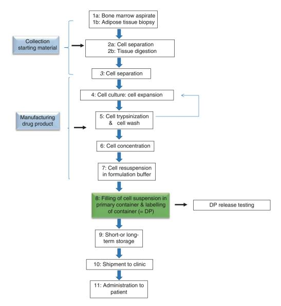
Figure 17.17 Flow diagram of a manufacturing process for an off-the-shelf (allogeneic) or non-off-the-shelf (autologous or allogeneic) cell-based product based on adherent cells which do expand *ex-vivo*, such as MSCs
