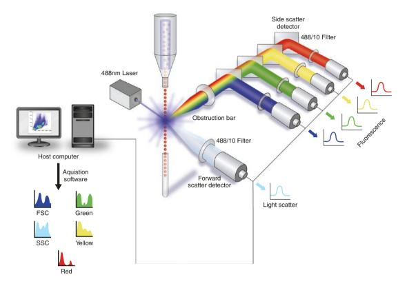
Figure 17.23 Schematic view of a flow cytometer. Scattered and emitted light signals are converted to electronic pulses, adapted from ThermoFisher Scientific. http://www.thermofisher.com/nl/en/home/life-science/cell-analysis/cell-analysis-learning-center/molecular-probes-school-of-fluorescence/flow-cytometry-basics/flow-cytometry-fundamentals/how-flow-cytometer-works.html#overview
