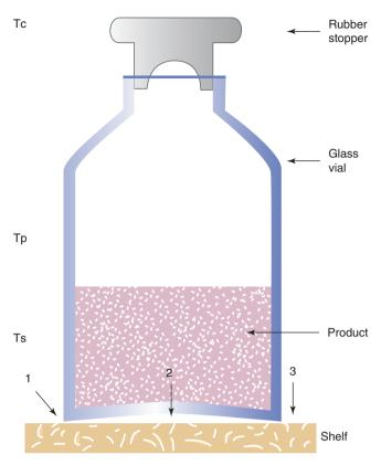
**Figure 5.10** Heat transfer mechanisms during the freezedrying process: (1) Direct conduction via shelf and glass at points of actual contact. (2) Gas conduction: contribution heat transfer via conduction through gas between shelf and vial bottom. (3) Radiation heat transfer. Ts shelf temperature, Tp temperature sublimating product, Tc temperature condensor. Ts > Tp > Tc
