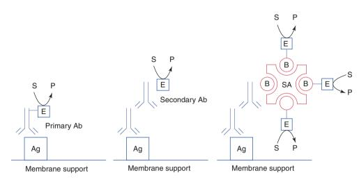
Figure 3.9 ■ Common immunoblotting detection systems used to detect antigens (protein of interest). Ag, on membranes. Abbreviations used: *Ab* antibody, *E* enzyme, such as horseradish peroxidase or alkaline phosphatase, *S* substrate, *P* product, either colored and insoluble or chemiluminescent, *B* biotin, *SA* streptavidin
