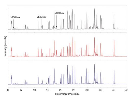
**Figure 3.13** A RP-HPLC peptide map of a MAB showing the oxidation of individual methionine residues (indicated by arrows). Top trace shows the peptide map of a non-oxidized protein sample, middle trace—sample oxidized using  $H_2O_2$  and bottom—sample to which  $H_2O_2$  and an antioxidant have been added
