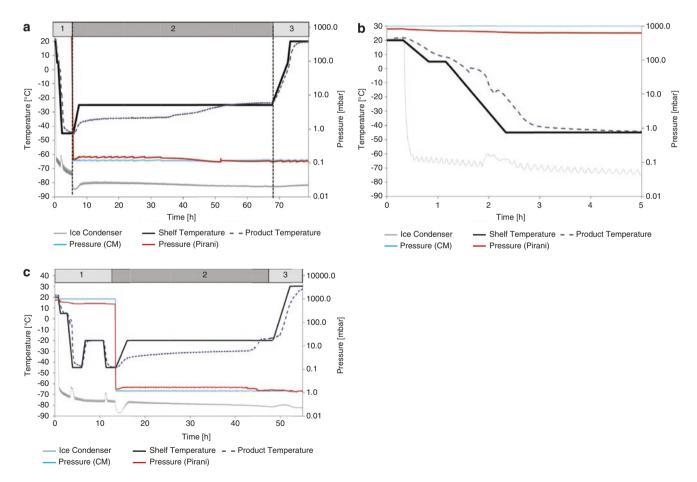
**Figure 5.7 (a)** Example of freeze-drying showing shelf temperature, product temperature, pressure (by Pirani and CM and ice condenser temperature. 1 = freezing stage, 2 = primary drying stage, 3 = secondary drying stage. See the text for explana-
