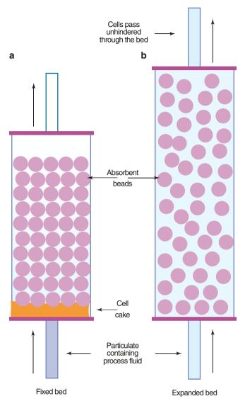
Figure 4.7 ■ Comparison between (a) a packed bed and (b) an expanded bed (adapted from Chase and Draeger 1993)
