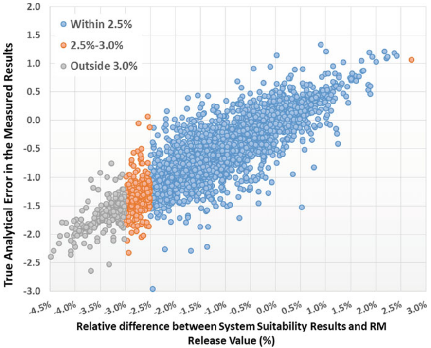
Fig. 7 Simulation results of analytical error in measured drug substance results versus in system suitability results
