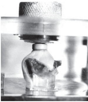
Figure 15.18 A device to measure the force of detachment of tablets or capsules from porcine oesophageal tissue, used to determine the values given in Fig. 15.19.
