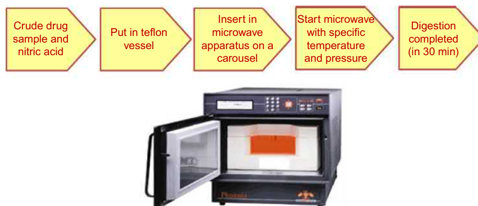
FIG. 4.12 Dry ashing using a microwave muffle furnace.
