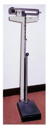
FIG. 3.2 Platform scale with height attachment.
