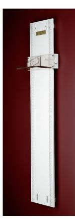
**FIG. 3.5** Device used to measure height of a child. (Courtesy Perspective Enterprises, Portage, MI.)
