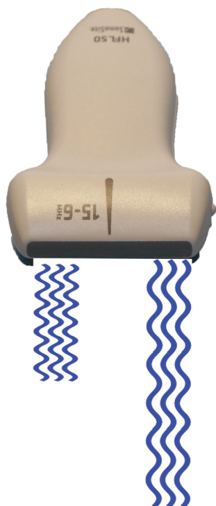
Figure 1-3 To achieve the best axial (vertical) resolution, one should use the highest frequency possible. This reduces the wavelength of the sound waves and makes discrimination of small structures possible. The trade-off is poor tissue penetration. The short-wavelength, high-frequency sound waves dissipate more energy, leading to greater attenuation (i.e., less tissue penetration).
