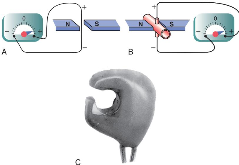
**Figure 14-4.** Flowmeter of the electromagnetic type, showing generation of an electrical voltage in a wire as it passes through an electromagnetic field (A); generation of an electrical voltage in electrodes on a blood vessel when the vessel is placed in a strong magnetic field and blood flows through the vessel (B); and a modern electromagnetic flowmeter probe for chronic implantation around blood vessels (C). N and S refer to the magnet's north and south poles.
