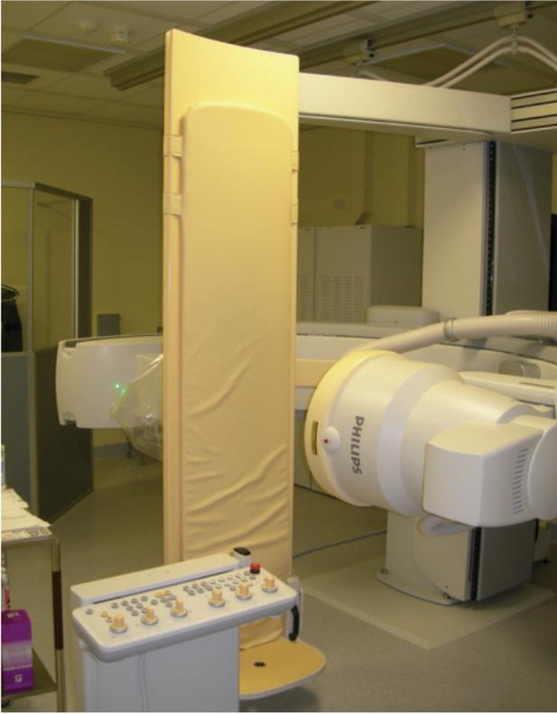
**Fig. 20.3** A typical fluoroscopy room set up for an upper gastrointestinal barium examination.
