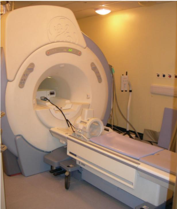
**Fig. 20.2** A typical MRI scanner. Note the absence of metal in the room (oxygen cylinder, etc.). A 'coil' is shown within the scanner.
