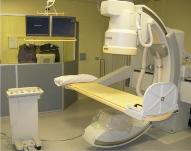
**Fig. 20.4** A typical fluoroscopy room set up for an upper gastrointestinal barium examination.
