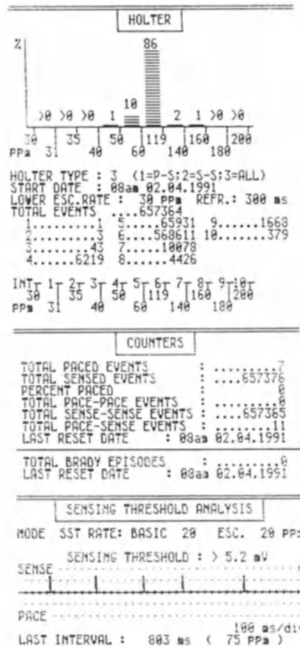
Fig. 7.8. Statistical information a Statistics offered by the Vitatron Diamond pacemaker. The main information consists of a count of ventricular extrasystoles and of abnormal atrial rhythms
