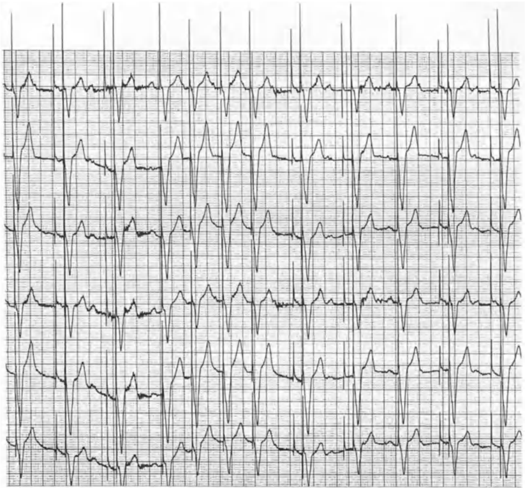
Fig. 8.51. Intermittent atrial sensing failure during exercise at an atrial sensitivity of 0.5 mV, whereas sensing was flawless at 3.5 mV at rest
