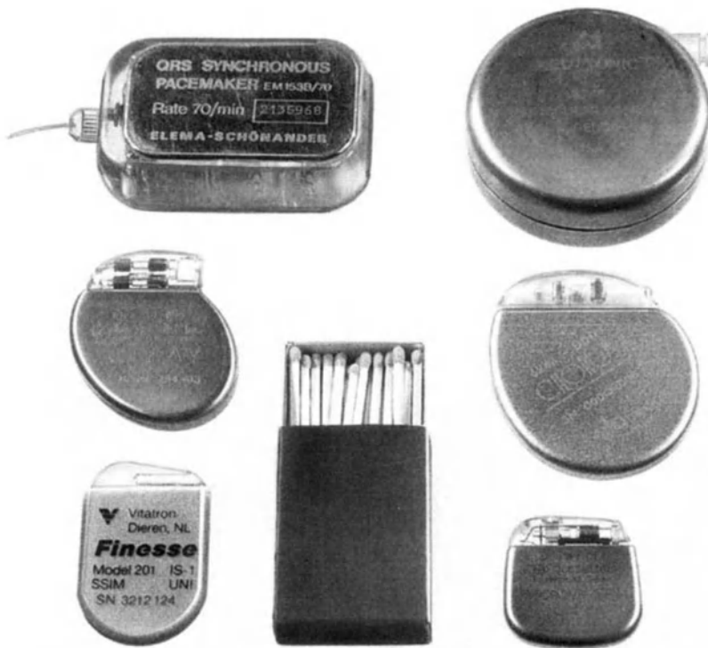
Fig. 3. Size changes of the implantable pacemaker over the course of time: two historic pacemakers ( upper row ), modern dual chamber pacemakers ( middle row ), and „Mini“ single chamber pacemakers ( lower row ); matchbox provided for size comparison
