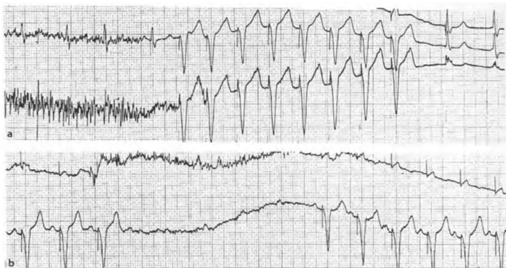
Fig. 7.1. Myosignal inhibition of the pacemaker must be systematically looked for a Sensing of myosignals by the atrial channel causing rapid ventricular pacing because of the interpretation of the myosignals as being of atrial origin b Myosignal sensing by the ventricular channel resulting in complete inhibition of pacing
