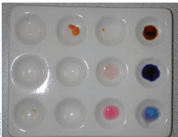
FIGURE 6 Examples of presumptive color tests for drugs. The pink reagent is cobalt thiocyanate and in the lower right is this reagent combined with cocaine. Note the shiny solid that forms, an ion/pair complex. The upper tier of tests consist of the Marquis reagent added to methamphetamine (right) and amphetamine (left). The middle well in the right column contains oxycodone and Marquis reagent.
