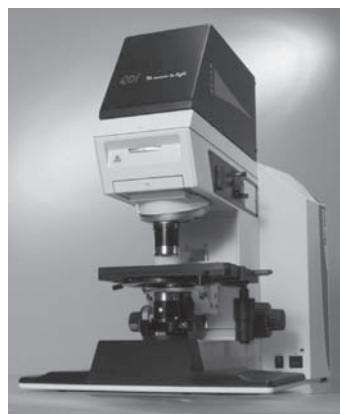
FIGURE 50 A commercial microscope base with a UV/VIS/NIR spectrophotometer detector and imaging system. Photo courtesy of Dr. Paul Martin, Criac Technologies.
