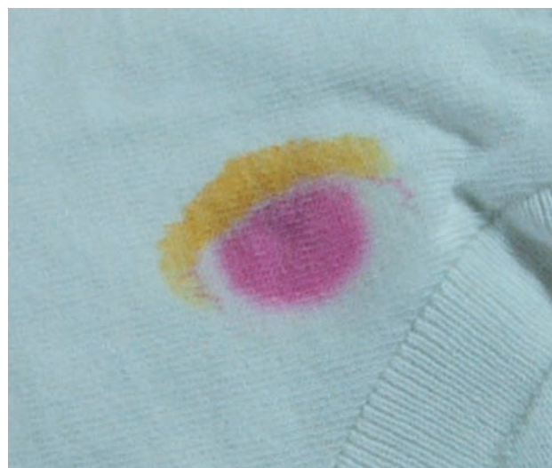
FIGURE 7 A bullet hole treated with sodium rhodizonate. The pink color indicates the presence of lead.
