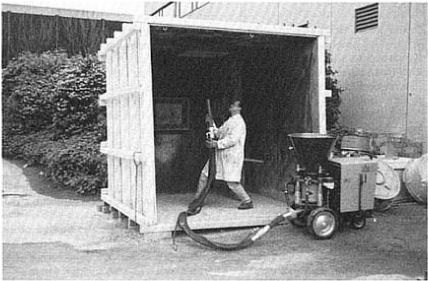
Fig. 5—Dry-mix shotcrete equipment and rebound chamber presently in use at UBC.
