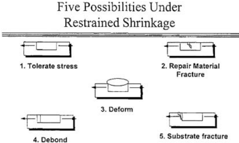
Fig. 2. A detailed diagram of what induced stress will produce in each of the following situations.
