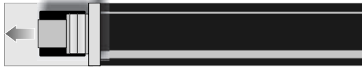
FIGURE 11.13 Formation of streaks or mixture pulling due to incorrect setup of paver screed segments.
