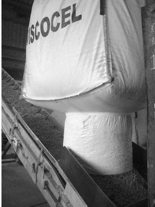
FIGURE 4.8 Dosing method of granulates—emptying a big-bag onto a conveyor belt. (Photo courtesy of Excel Industries Ltd., U.K.)
