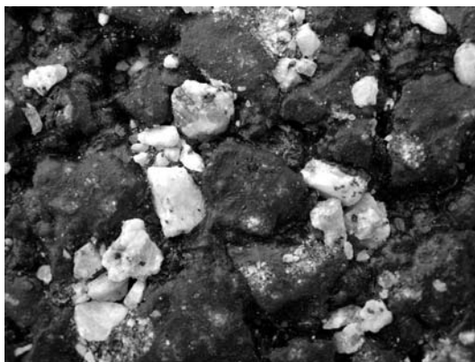
FIGURE 10.14 Gritting particles among SMA coarse aggregates. (Photo courtesy of Krzysztof Błażejowski.)
