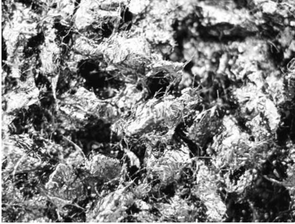
FIGURE 4.3 Plastic fibers can be an SMA stabilizer but must be used at a high-addition rate. The photo shows an SMA mix with 0.6 % (m/m) of polypropylene fibers. (Photo courtesy of Halina Sarlińska.)
