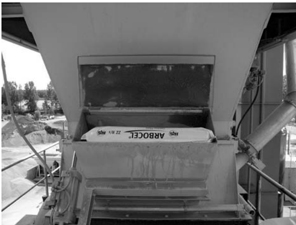
FIGURE 9.9 Manual charging box with a motor-driven chute. (Photo courtesy of Bartosz Wojczakowski.)
