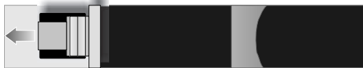
FIGURE 11.15 Area of an uncompacted cool mixture during a paver standstill (a zone of cooling mixture that is inaccessible to rollers).
