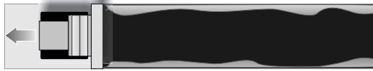
FIGURE 11.19 Manually corrected edges of a working lane with cooler temperatures and higher porosity.
