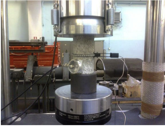
Figure 2.16 Experimental setup of the compression test on the concrete specimen.
