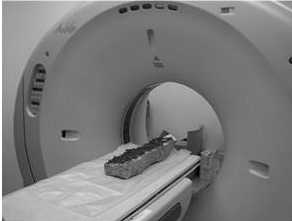
Figure 1.7 A general view of the helical computed tomography machine and a sample.
