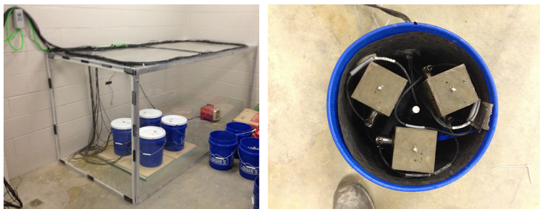
Figure 11.6 Test setup. Controlled temperature chamber (left) and specimens placed in 100% relative humidity buckets (right) (ElBatanouny, Jones, et al., 2014).
